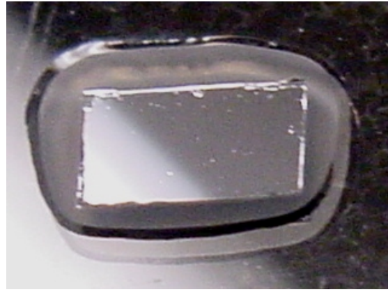
Figure 10. Device after it has been cleaned. The debris on the surface is due to dust that immediately bonds to the surface after cleaning.
