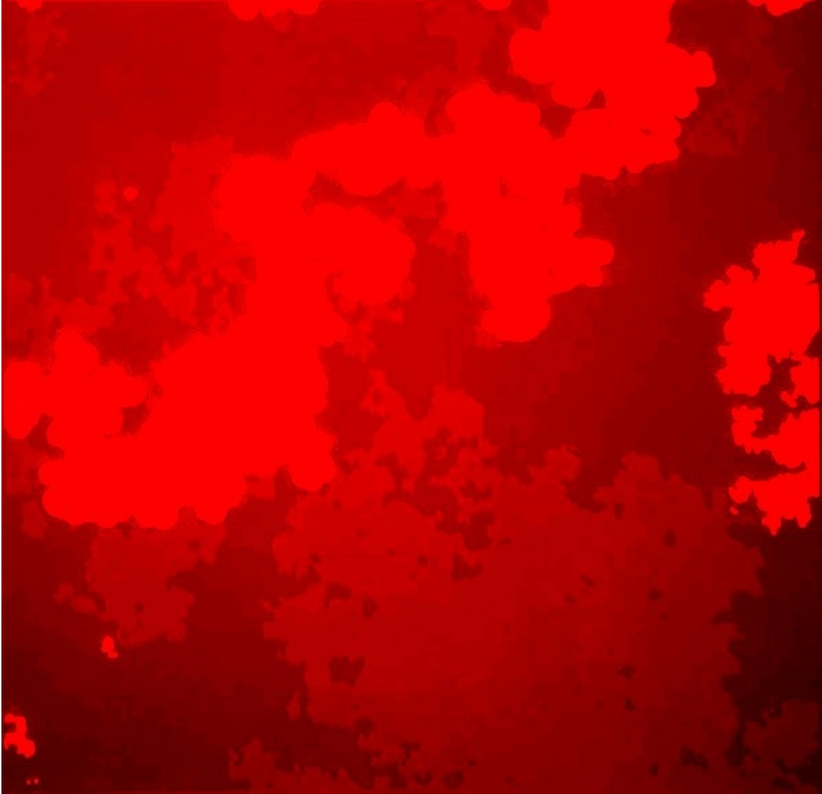
Figure 33. Micromodel from Figure 1 filled with nitrogen gas (brightest areas) and decane. The darkest regions are inaccessible to fluid.
