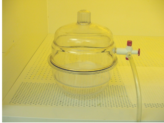
Figure 3. Desiccator used to remove bubbles from the epoxy.
