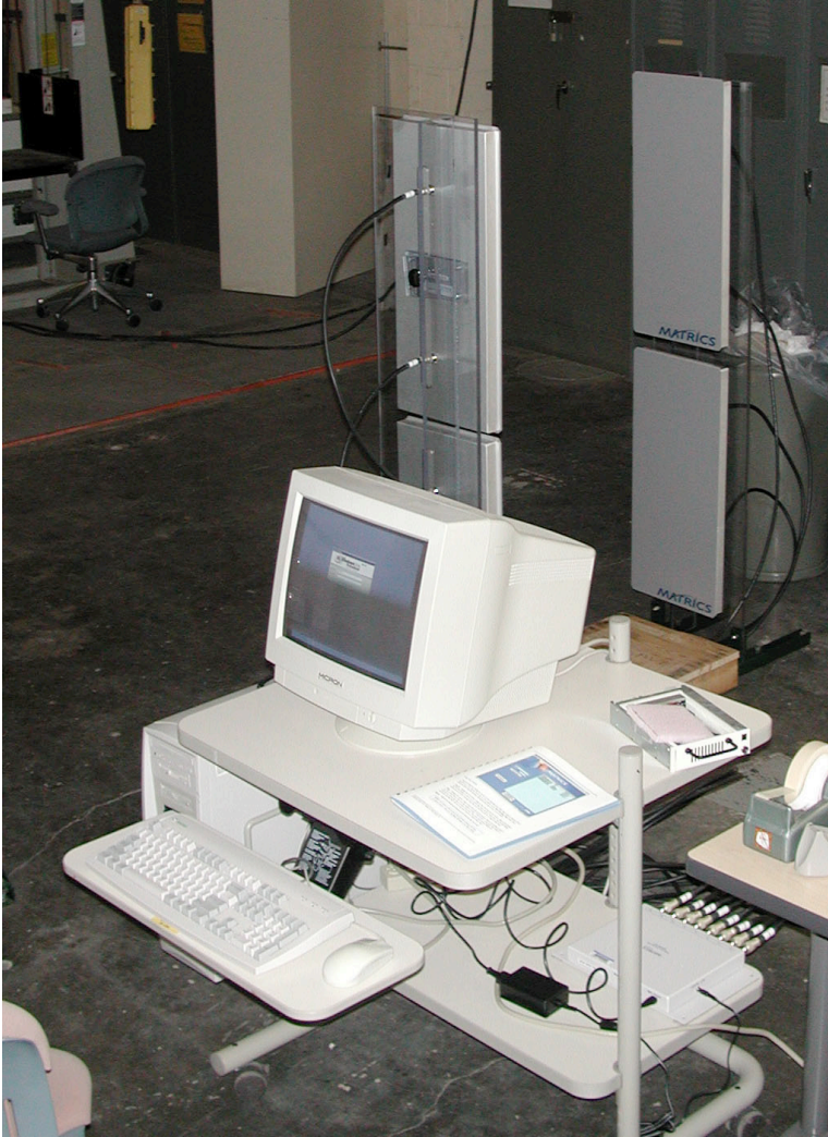
Figure A2-7. A lateral view shows the gate antennae for System B behind the standalone PC host in the foreground.
