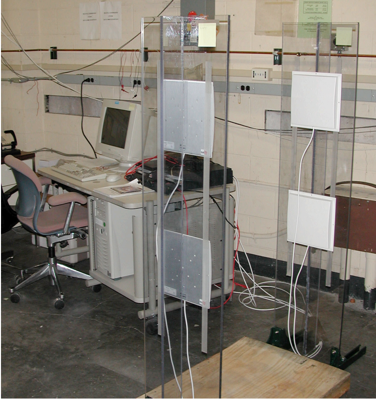
Figure A2-9. The image shows the arrangement of the gate antennae for System C.
