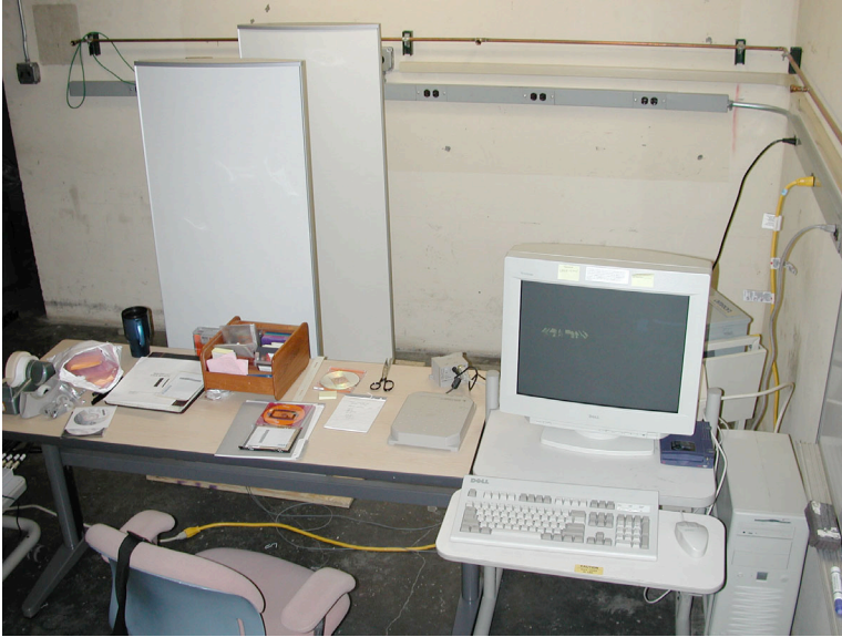
Figure A2-3. The gate antennae for System A (background) are connected to the standalone PC host, shown in the foreground.
