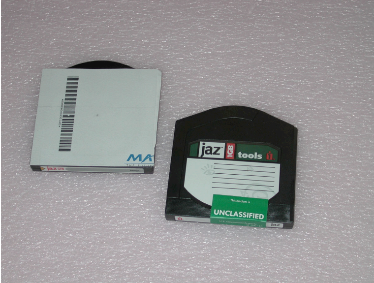
Figure A2-5. A Matrics model DDS-001 tag affixed to a Jaz disk.
