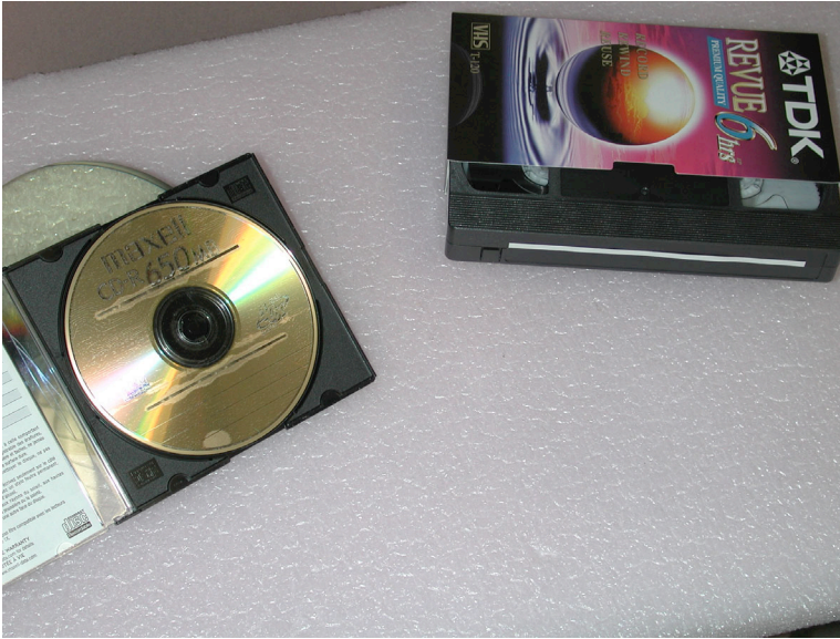
Figure A2-10. The image shows a 3M model DCD-2 tape affixed to a CD-ROM in the jewel case, and a 3M model DVM-1 strip tape affixed to a VHS videocassette in the sleeve.
