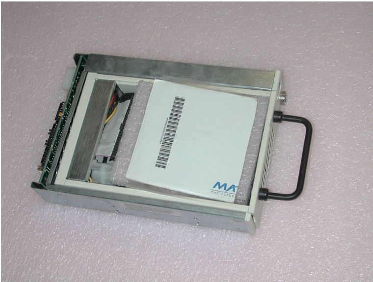
Figure A2-6. The Matrics model DDS-001 tag is affixed to a removable hard drive case, with a half-inch polyurethane foam spacer between drive and tag.
