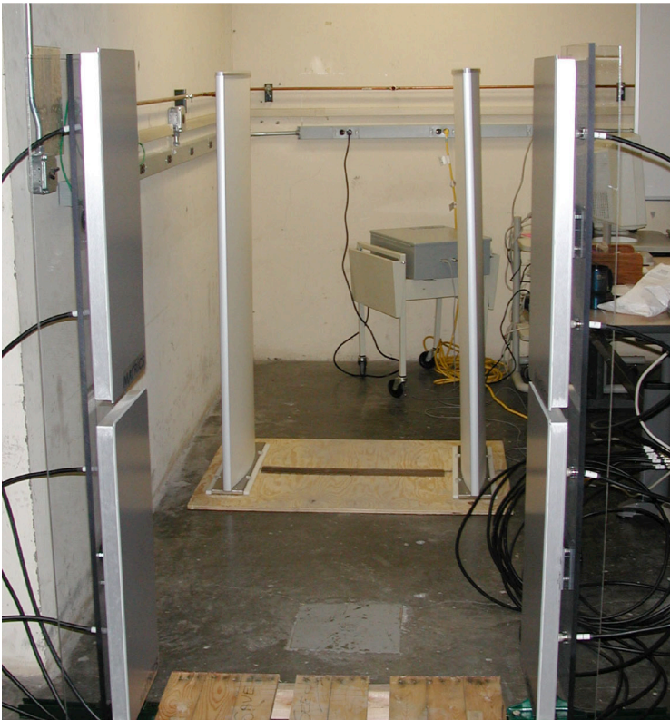
Figure A2-4. A runway view of the portal antennae shows System A in the background, and System B in the foreground.
