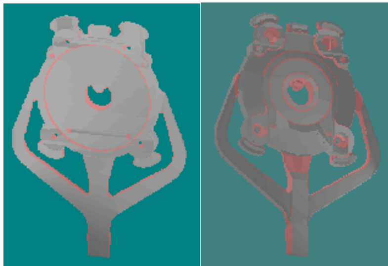
(a) The photograph of the ejection marks obtained from the real casting product.
