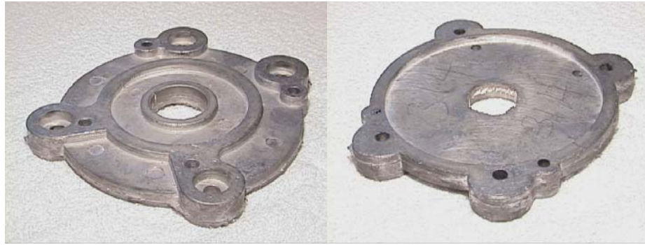
(a) The photograph of the ejection marks obtained from the real casting product.
