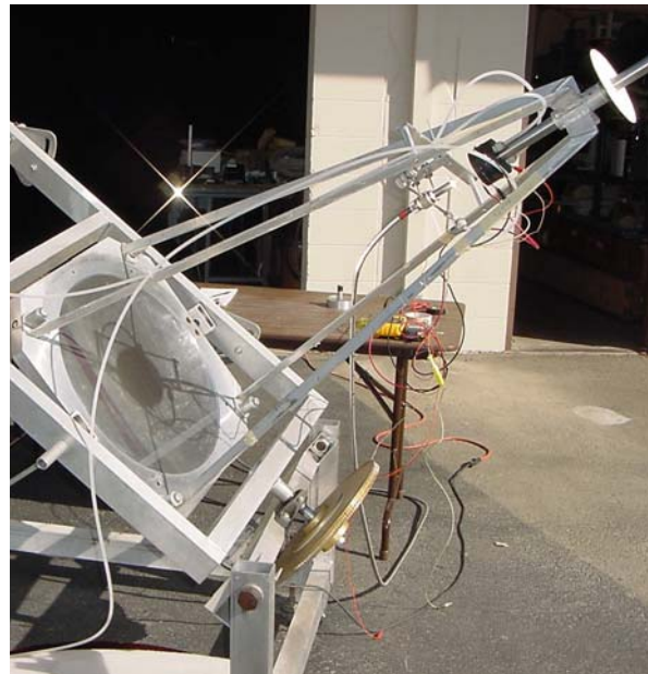
Figure 2. Experimental facility for GaSb cell performance characterization tests for solar spectra
