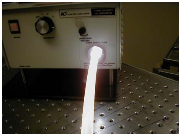
Fig. 1. Photograph of 3M light guide pressed into tapered aperture of light source
