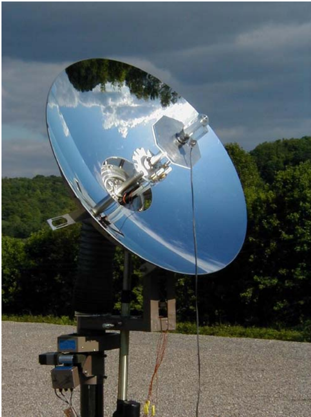
Fig. 1. Solar tracker and collector system partially populated with four waveguides
