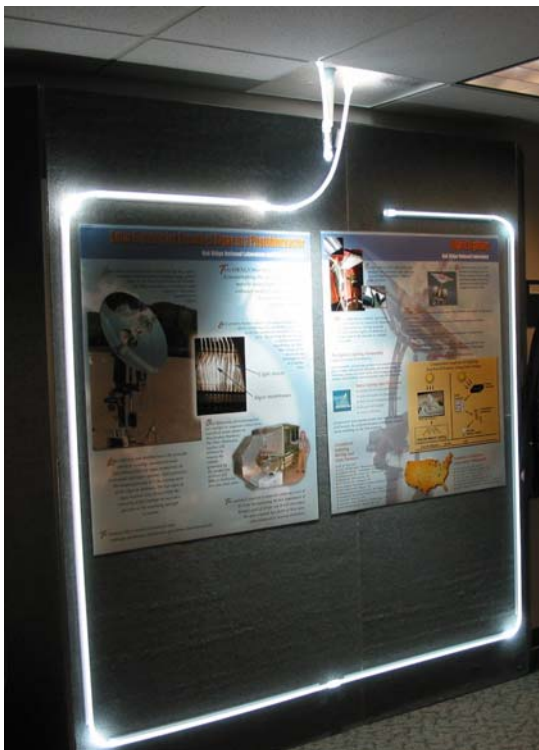
Fig. 3. Demonstration of fiber optic transporting day light from roof mounted collector/receiver
