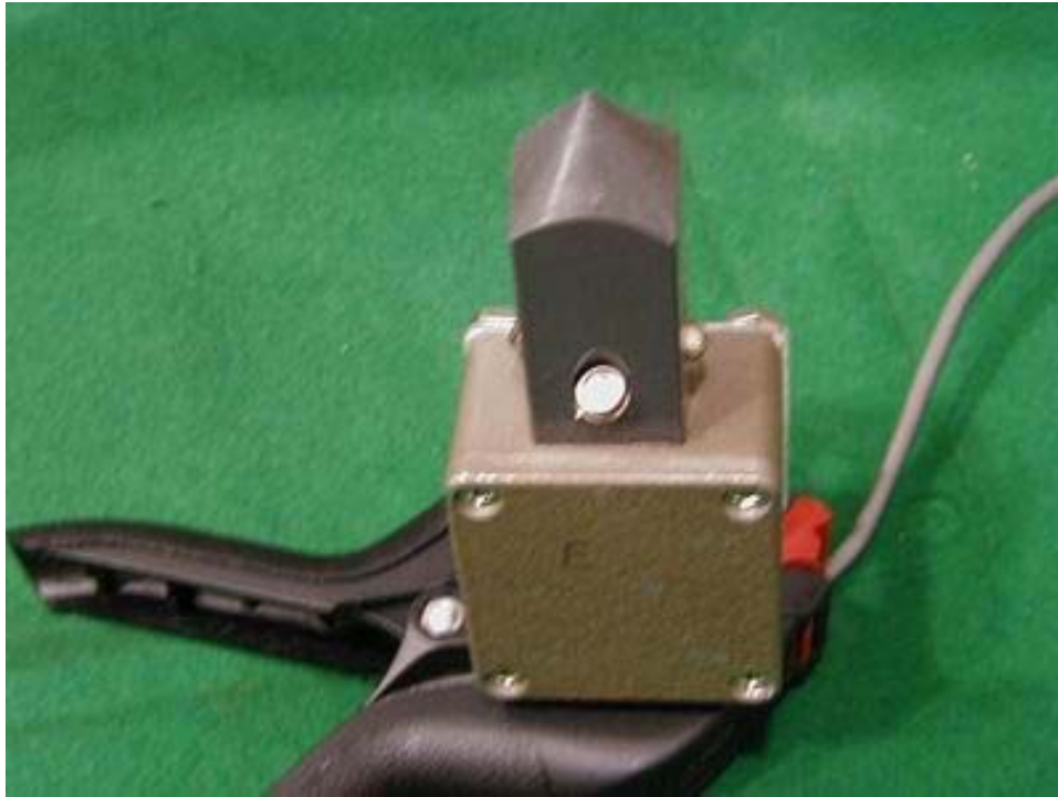
Figure 4. Optical Sun Sensor device used to provide feedback to the electronics control system.
