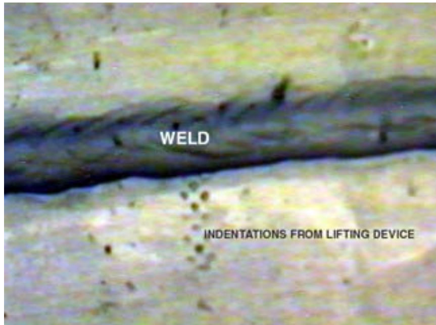
Figure D-5. Areas of mechanical damage from initial tank construction (PD03-0029-06). 5
