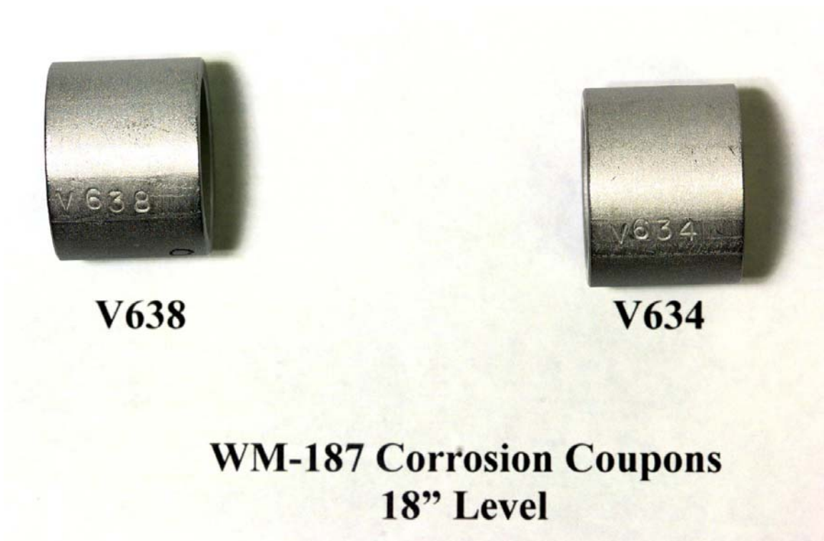
Figure C-23. Tank WM-187 coupons at the 45-cm (18-in.) level after 38.6 years of exposure (PD01-0406-16).
