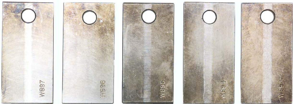
WM-183 (BOTTOMS) TYPE 304L SS - 11.5 Yr EXPOSURE
