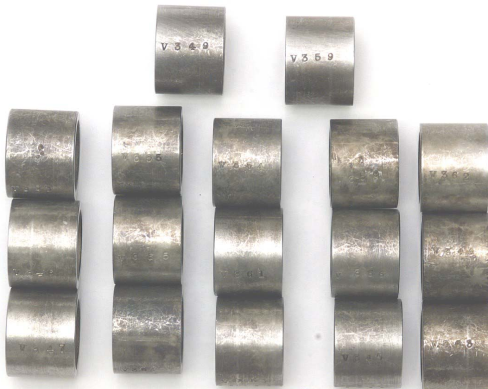
WM-183 (18 IN LEVEL) – TYPE 304L SS 38.5 YEARS EXPOSURE
