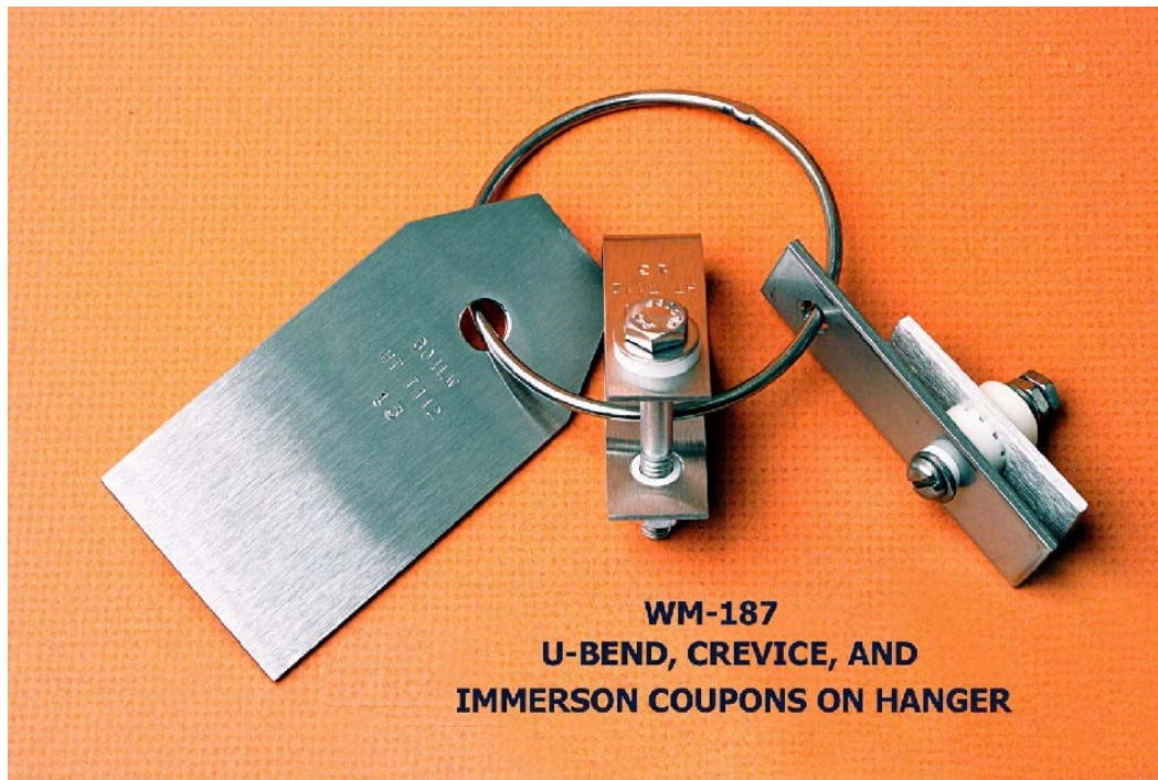
Figure C-35. Types of new corrosion coupons added to the 300,000-gal tanks during 2001 and 2002 (PD01-152-2-6). 9
