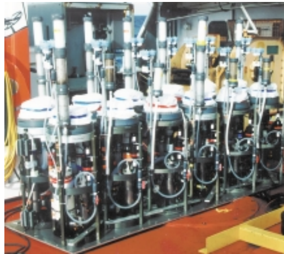
Fig. 3.5. The multiple unit large-volume in situ filtration system (MULVFS) allows the precise determination of properties of particulate matter that is needed for a systematic survey of ocean carbon inventory and for the evaluation of ecosystem function. MULVFS samples are large enough to meet the diverse needs of multiple research groups.
