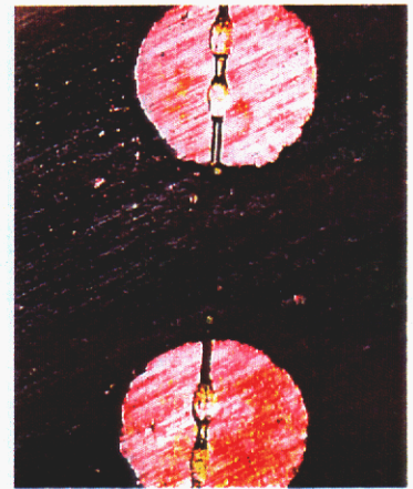
Figure 13. Microscope pictures of bare bridgewire detonators after applying 6A, 7A, and 8A, respectively.
