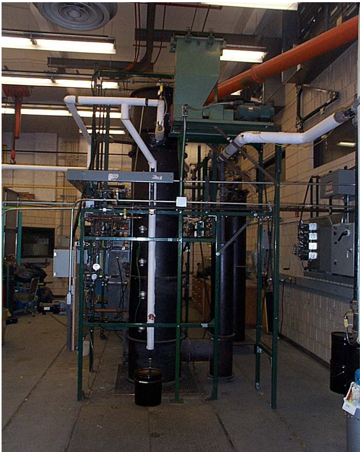
Figure 2. Down-flow reactor with biomass hopper, steam drain, and water jacket.
