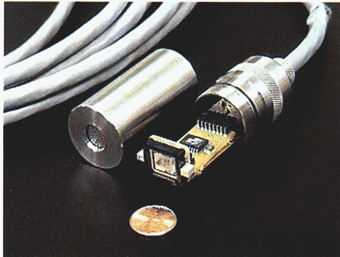
Figure 6. Integrated SAW probe for in-situ monitoring applications.
