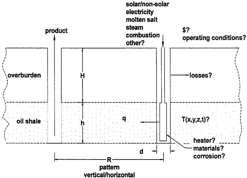
Figure 1. *In situ* heating method.
