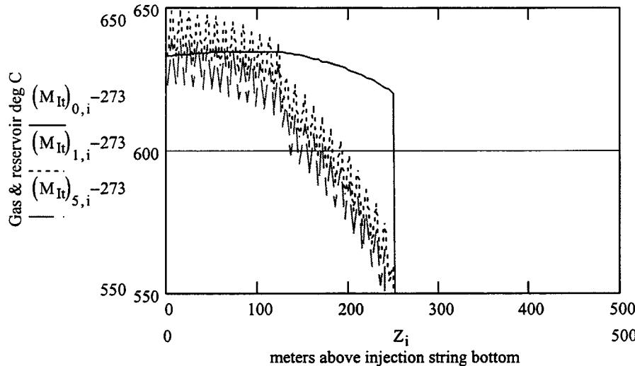
**Figure 29. Baseline DHC case 18000-hour magnified flue gas and casing temperatures with mid-depth 30% reduction in shale thermal conductivity over 32°.**
