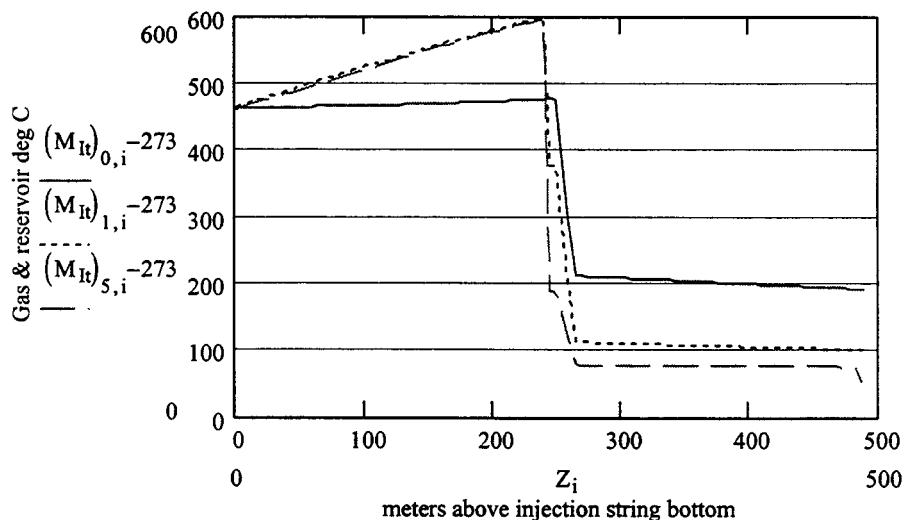
**Figure 24. Temperature of air and flue gas (solid and dotted lines) and casing (dashed line); base case, single DHC.**
