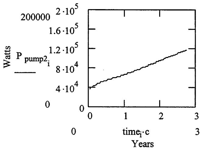
**Figure 23. Compressor power; base case, single DHC.**
