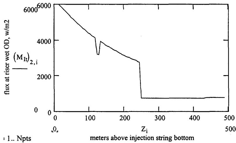
**Figure 11. Baseline case 80-hour radial heat flux with mid-depth 30% reduction in shale thermal conductivity over 32'.**
