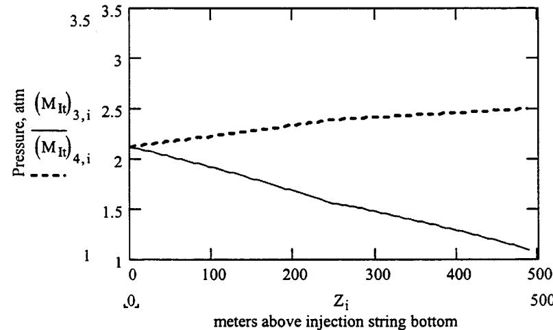
**Figure 22. Air and flue gas pressure; base case, single DHC, 33 months.**
