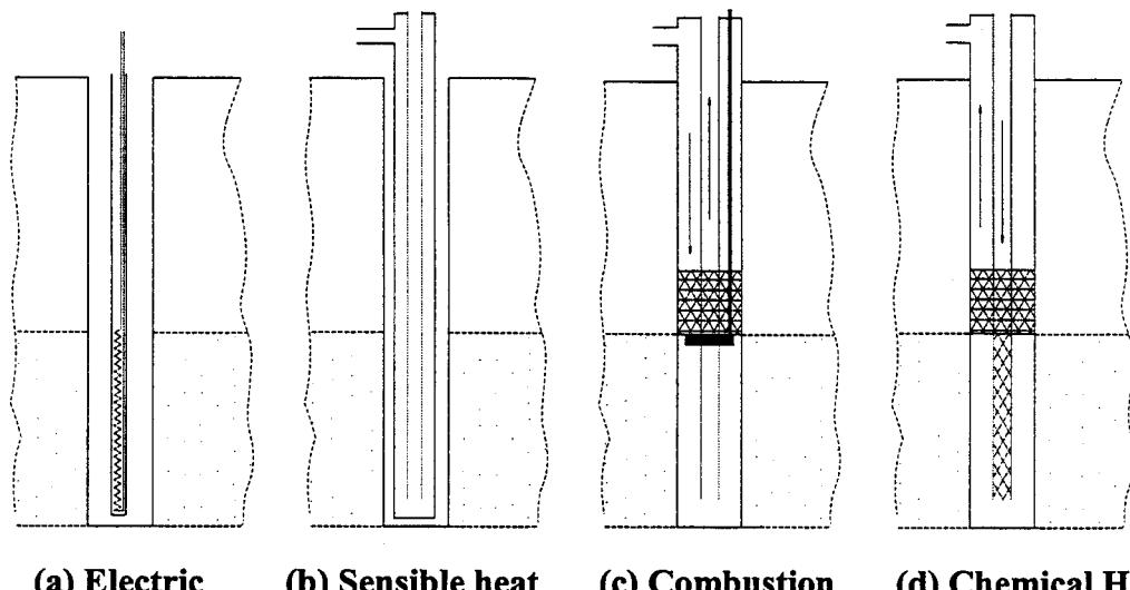
Figure 2. Shale heating concepts
