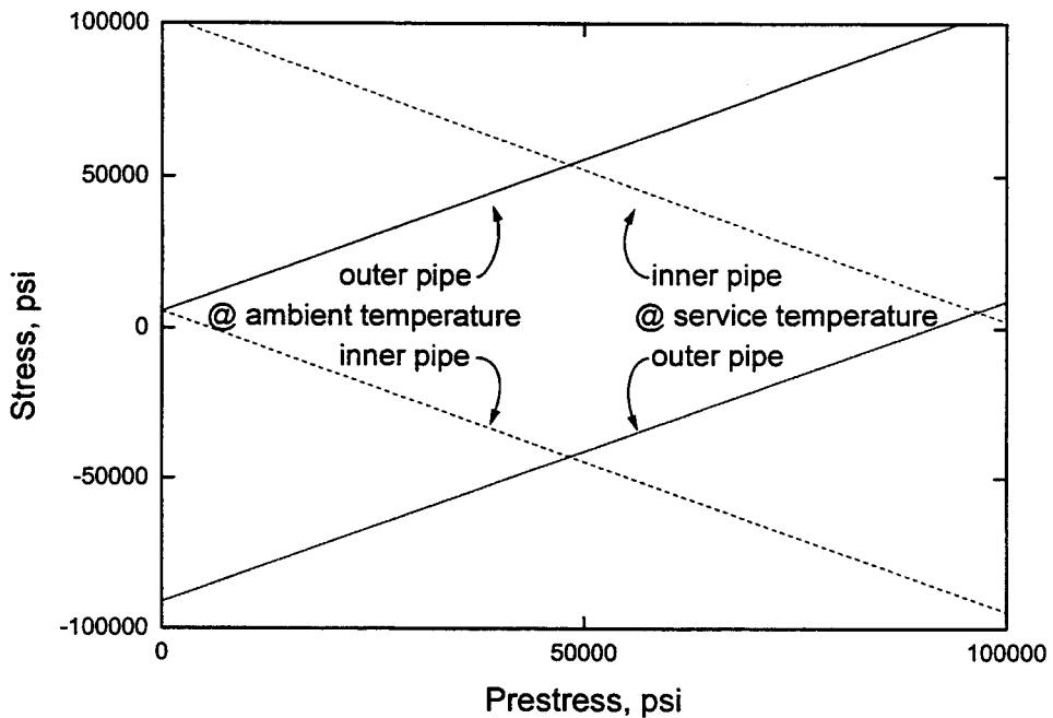
**Figure 4. Stresses as a function of pre-stress, for vacuum-insulated pipe**
