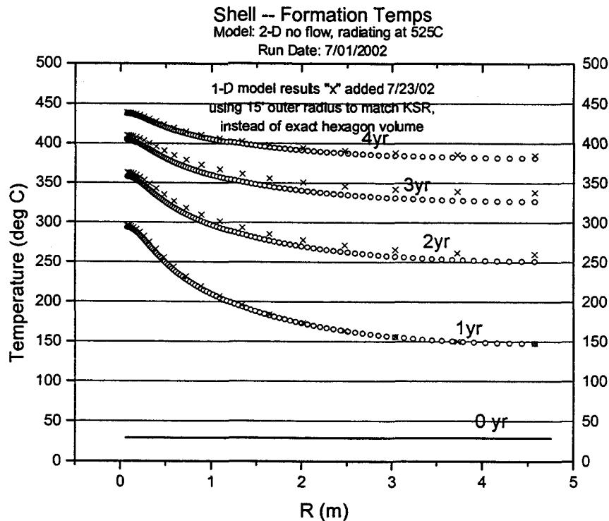
**Figure 6. Comparison of results from FEA (circles) and simple model (Xs) for the case of uniform-temperature radiant source cycling diurnally to simulate solar input.**
