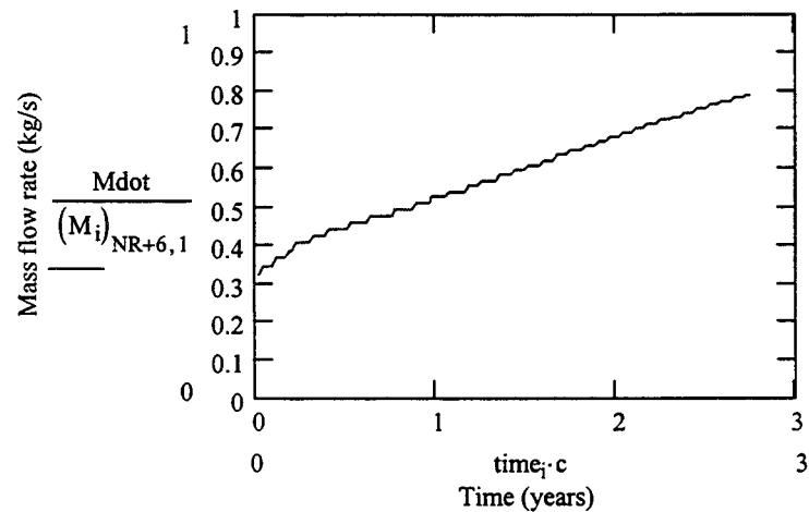
**Figure 21. Mass flow rate; base case, single DHC.**
