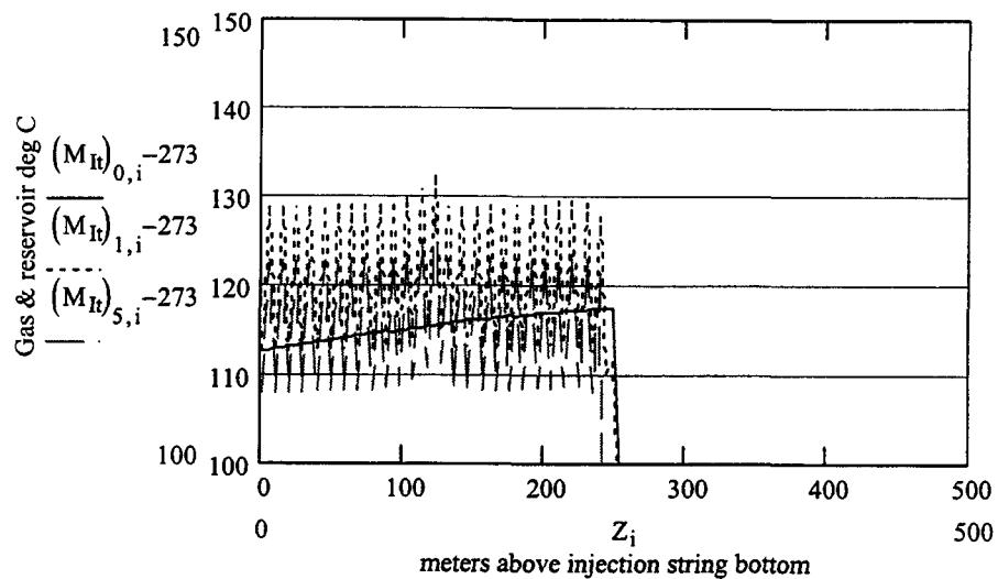
**Figure 27. Baseline DHC case 160-hour magnified flue gas and casing temperatures with mid-depth 30% reduction in shale thermal conductivity over 32'.**
