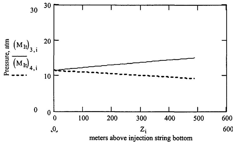
Figure 18. Case # 18 steam pressure distributions for a source pressure of 15 atm.
