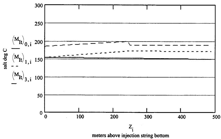
**Figure 13. Casing, riser, and downcomer temperatures, after 2 years of heat extraction.**
