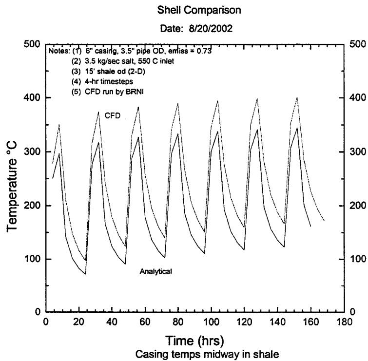
**Figure 7. Comparison of predictions of well-casing temperature from FEA and simple models for the conjugate problem, with diurnal molten-salt heat input.**
