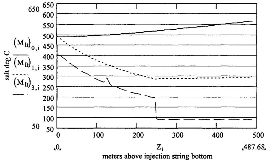
**Figure 10. Baseline case 80-hour salt and casing temperatures with mid-depth 30% reduction in shale thermal conductivity over 32'.**
