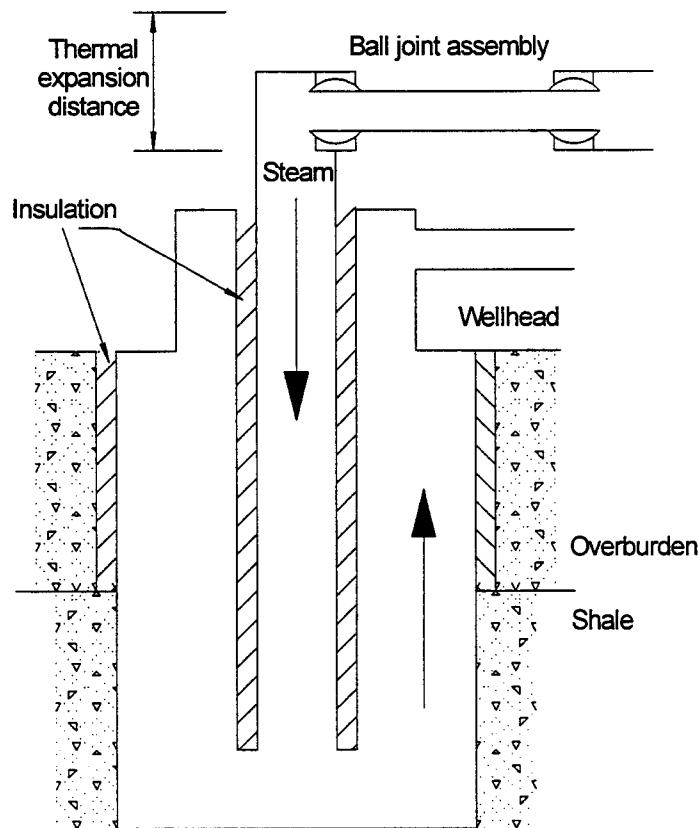
**Figure 17. Steam insulated tubing and well head**
