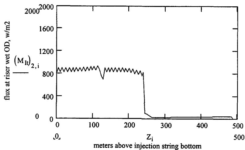
**Figure 28. Baseline DHC case 160-hour flue radial fluxes with mid-depth 30% reduction in shale thermal conductivity over 32'.**
