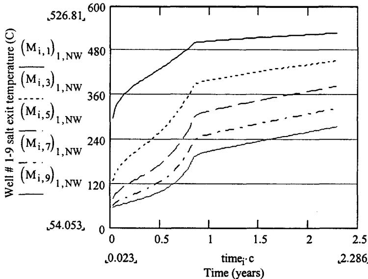
**Figure 16. Simulation of molten salt exit temperatures for 9 wells in series.**
