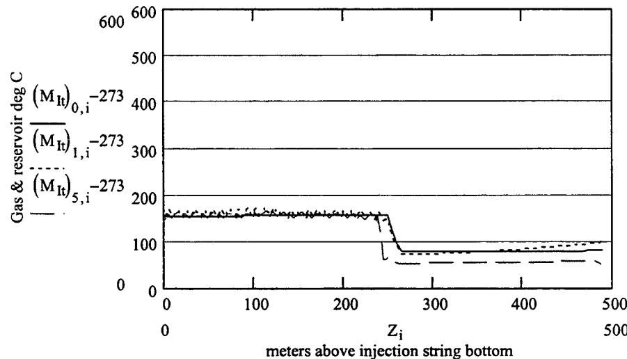
**Figure 26. Baseline DHC case 160-hour flue gas and casing temperatures with mid-depth 30% reduction in shale thermal conductivity over 32'.**
