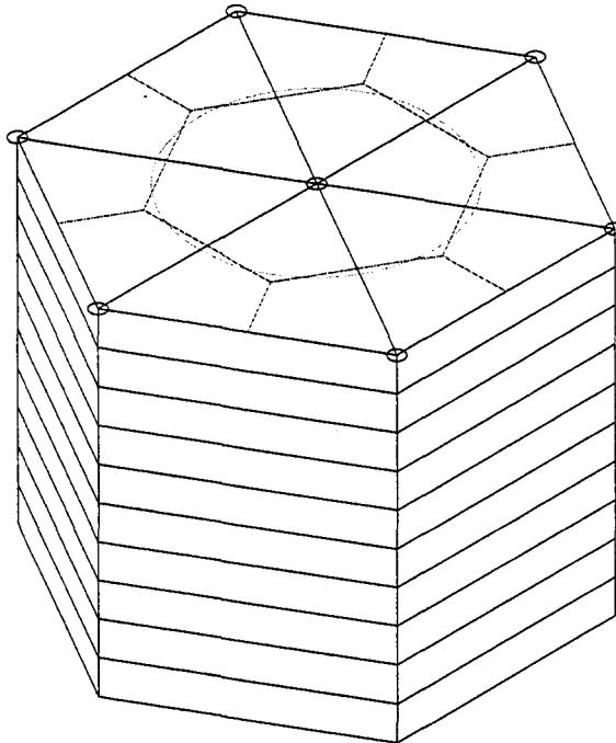
**Figure 5. Approximation of the geometry surrounding an injection well in a triangular pattern as cylindrical (hexagonal adiabatic boundary approximated as circular).**
