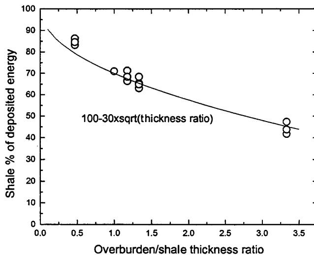
**Figure 9. Molten shale predicted efficiencies and their correlation.**
