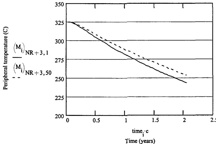
**Figure 15. Shale temperatures during heat extraction, at maximum radius, bottom & top of interval, vs time.**
