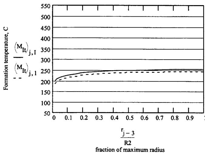
**Figure 14. Shale temperatures vs radius, bottom & top of interval, after 2 years of heat extraction.**
