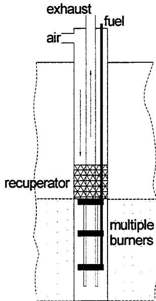
**Figure 20. Downhole combustor concept.**
