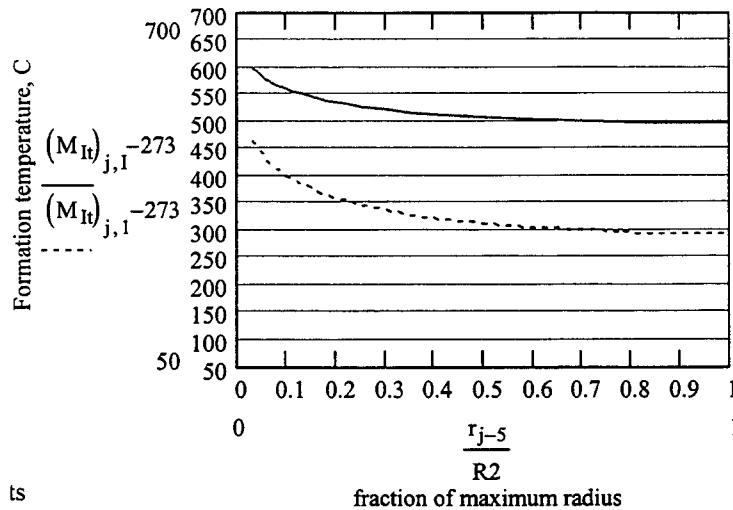
**Figure 25. Temperature of the shale near its top (solid line) and bottom (dotted line); base case, single DHC.**
