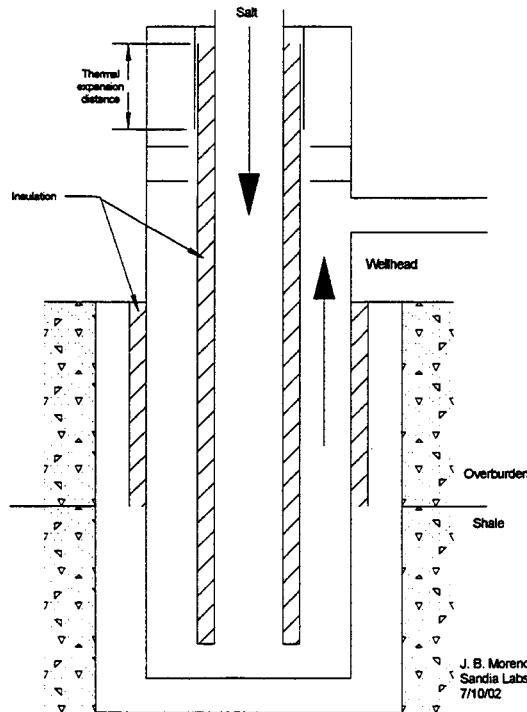
**Figure 3. Molten-salt insulated string and well-head concept.**
