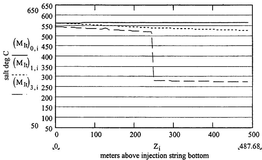
**Figure 12. Baseline case 18000-hour salt and casing temperatures with mid-depth 30% reduction in shale thermal conductivity over 32'.**
