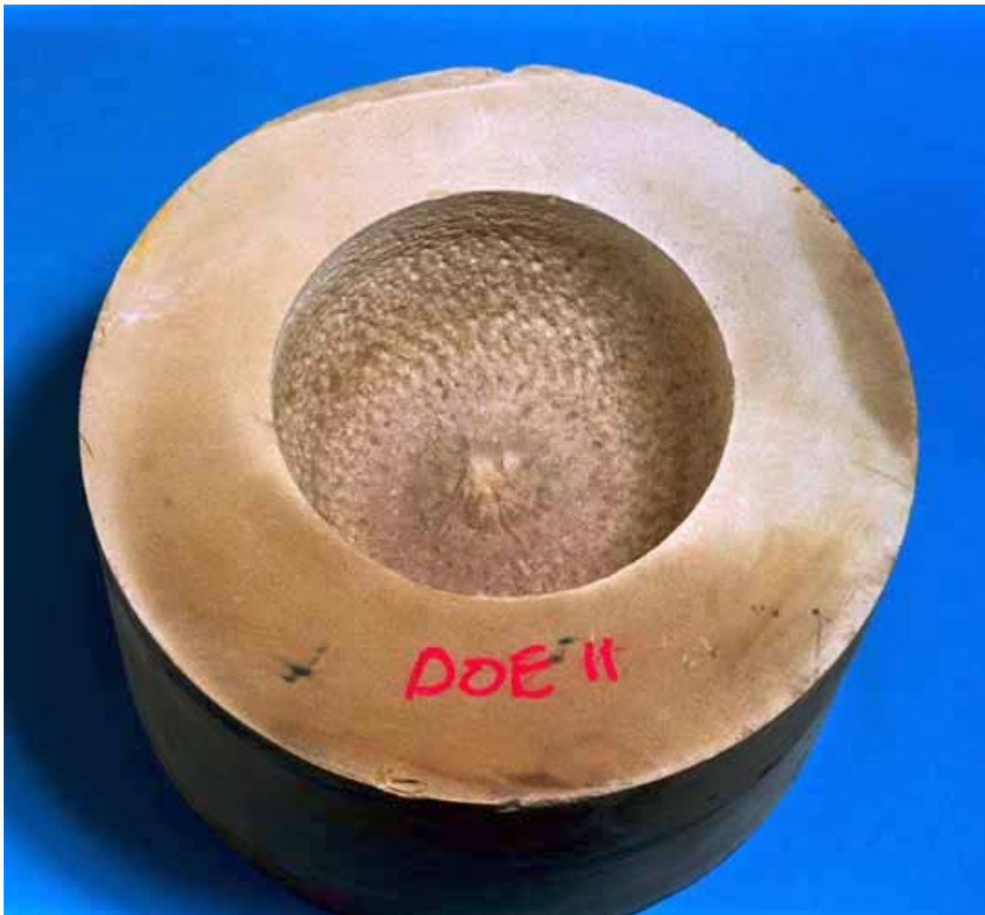
Bottomhole pattern from Novatek hammer / bit drilling in a Crab Orchard Sandstone sample
