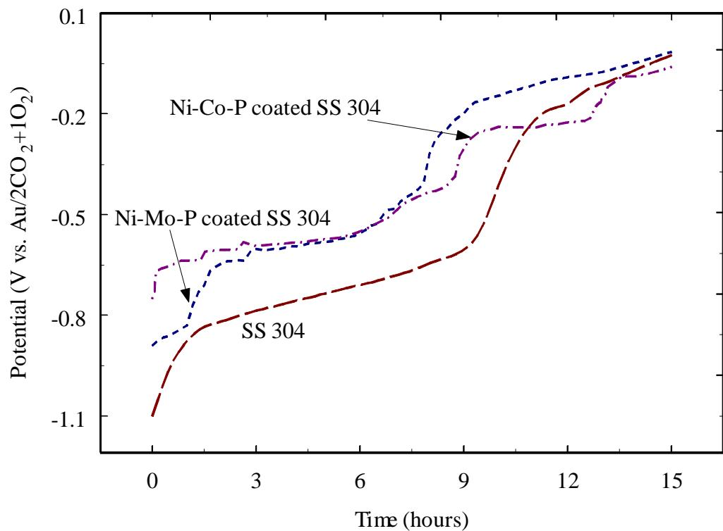
Figure 12. Open circuit potential response of bare and surface modified SS 304 as a function of exposure time in molten carbonate melt under cathode gas conditions. The potential is referenced to the oxygen reduction reaction happening on a gold electrode.
