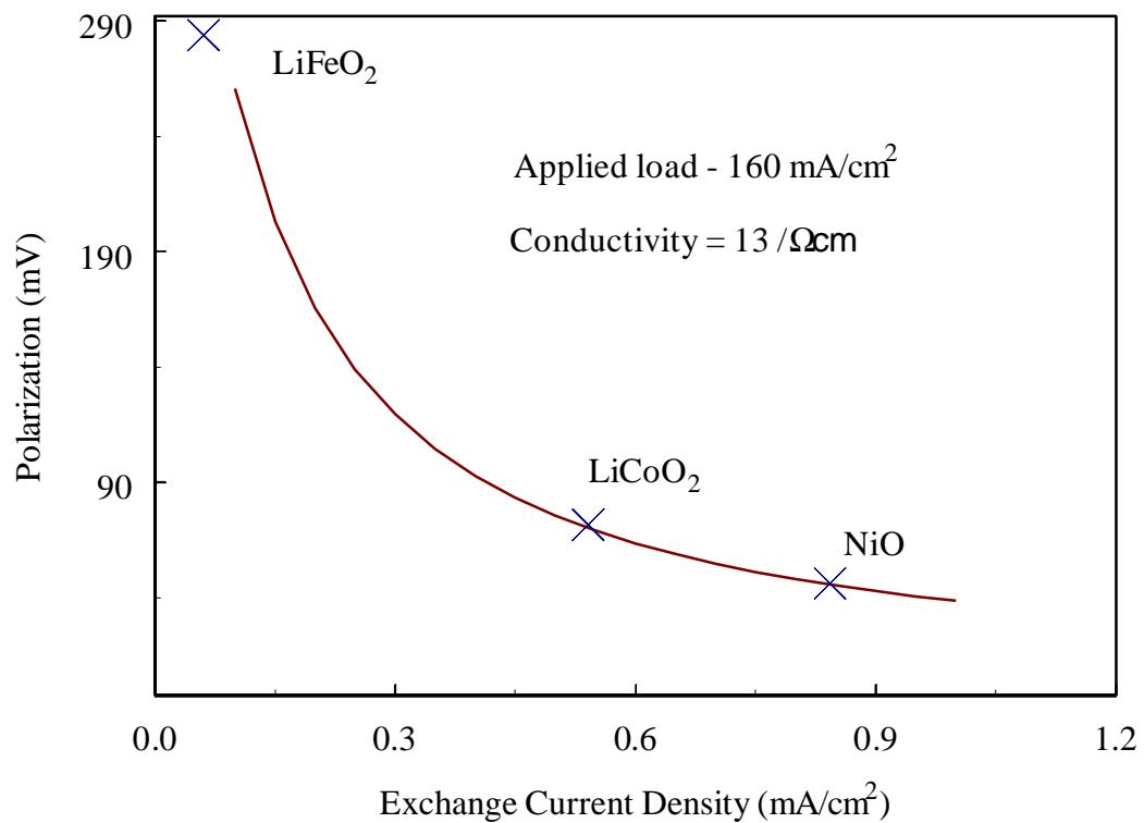
Figure 5. Cathode polarization plotted as a function of exchange current density. The electrode conductivity is  $13 \Omega^{-1} \text{cm}^{-1}$  and the applied load is  $160 \text{ mA/cm}^2$ .
