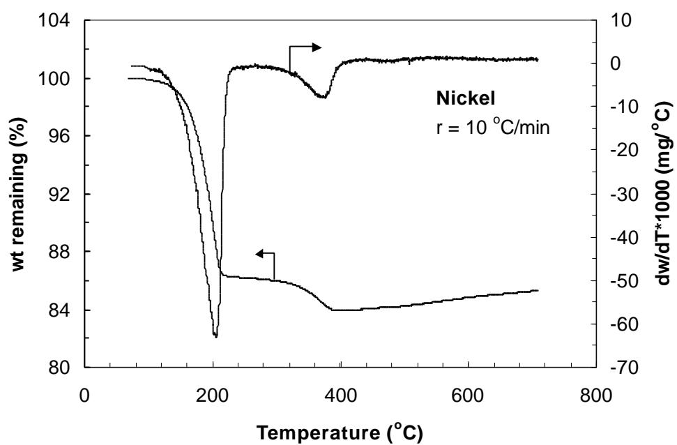
Figure 1. Thermo gravimetric analysis (TGA) of an aqueous nickel tape.
