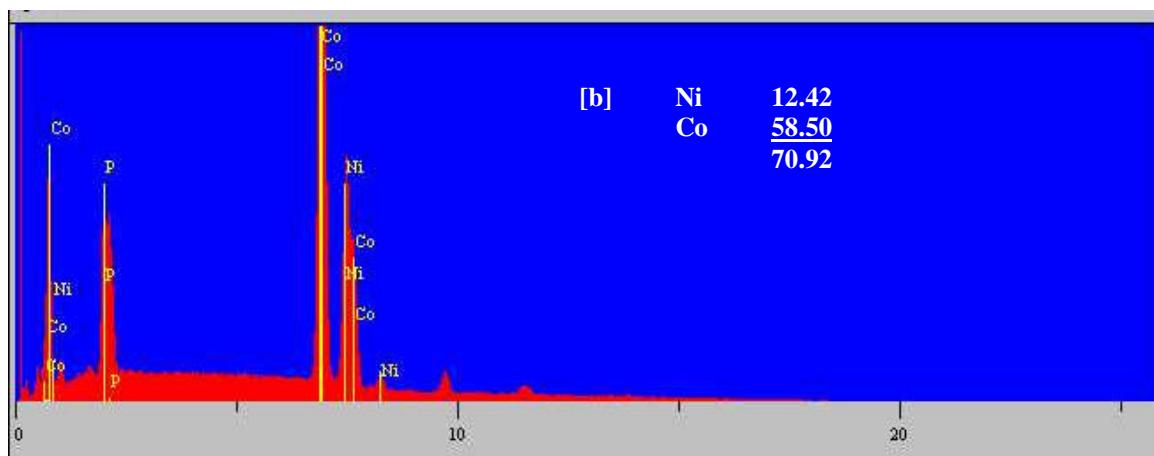
Figure 11. EDAX analysis done on cobalt encapsulated and bare nickel oxide cathodes after 72 hours (a) and 300 hours (b) of operation.
