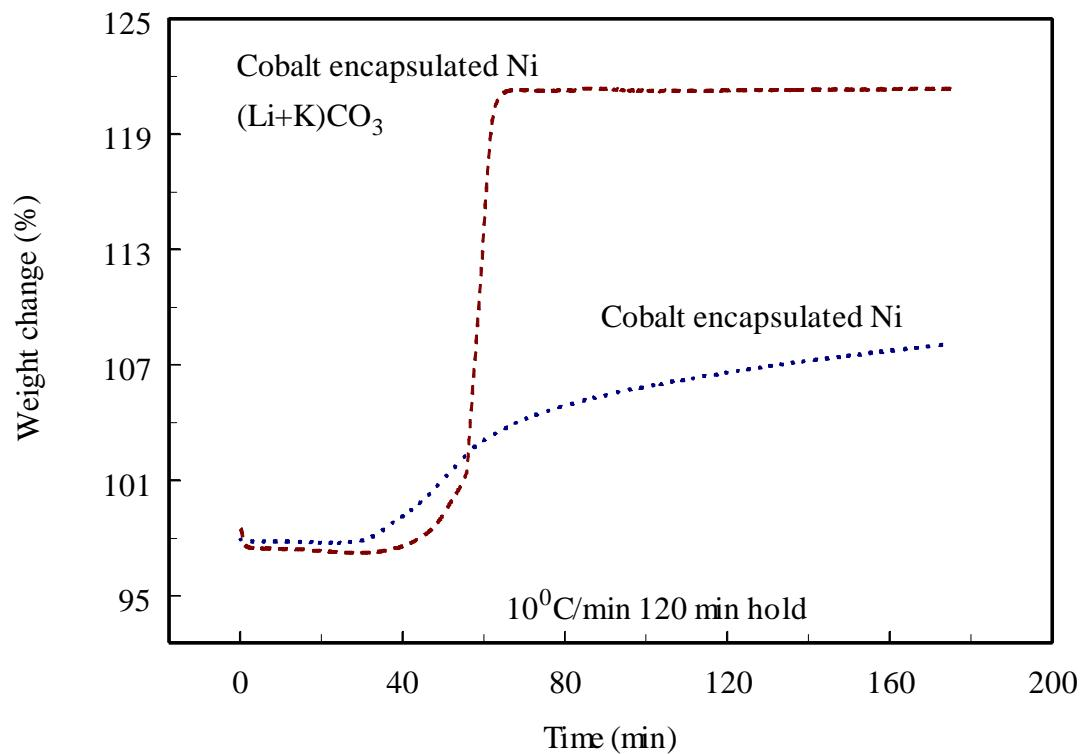
Figure 8b. TGA analysis of sintered cobalt encapsulated nickel tape under cathode gas conditions in the presence and absence of molten carbonate melt.
