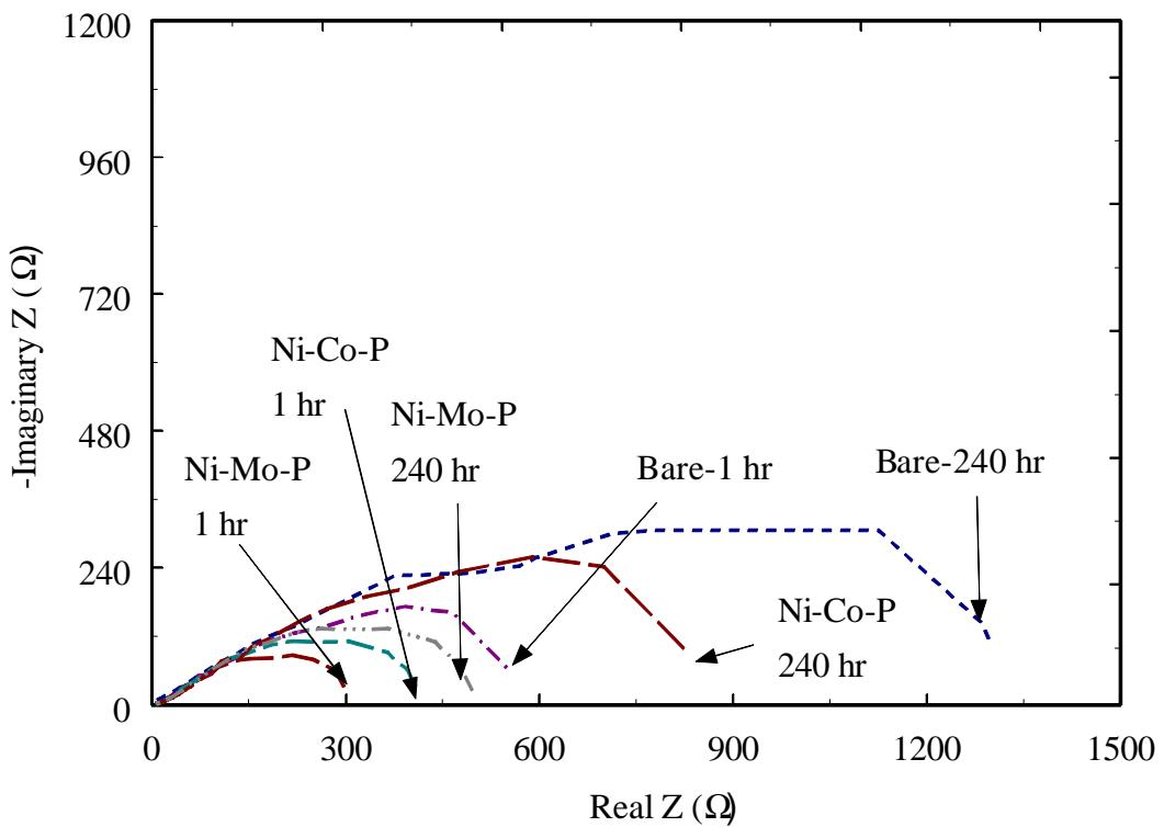
Figure 13. Nyquist plots of bare and surface modified SS 304 recorded after 1 hour and 10 days after immersion in molten carbonate melt under cathode gas conditions.
