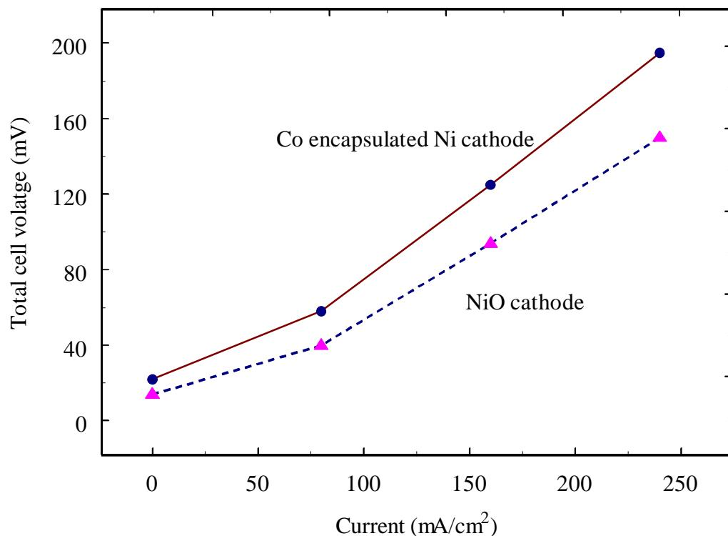
Figure 10. Comparison of cathode polarization behavior at different current loads for bare and cobalt encapsulated nickel cathodes.
