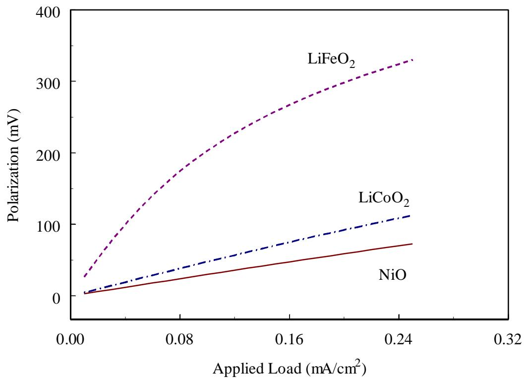
Figure 3. Cathode polarization curves simulated for different materials under various applied loads.
