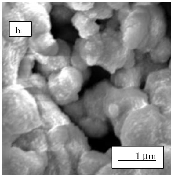
Figure 6. SEM photographs of bare (a, left) and cobalt microencapsulated (b, right) nickel electrodes obtained by tape casting and sintering.
