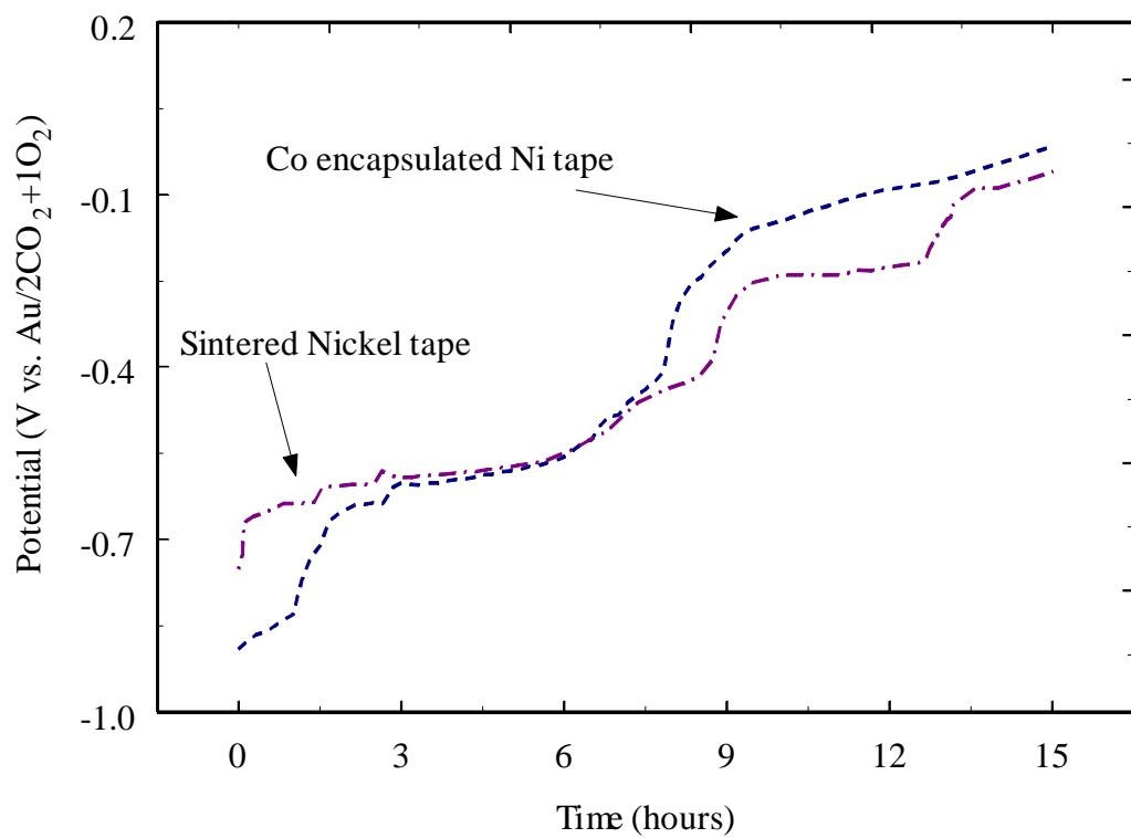
Figure 9. Open circuit potential as a function of time during the *in-situ* oxidation of bare and cobalt encapsulated nickel tapes under cathode gas conditions.
