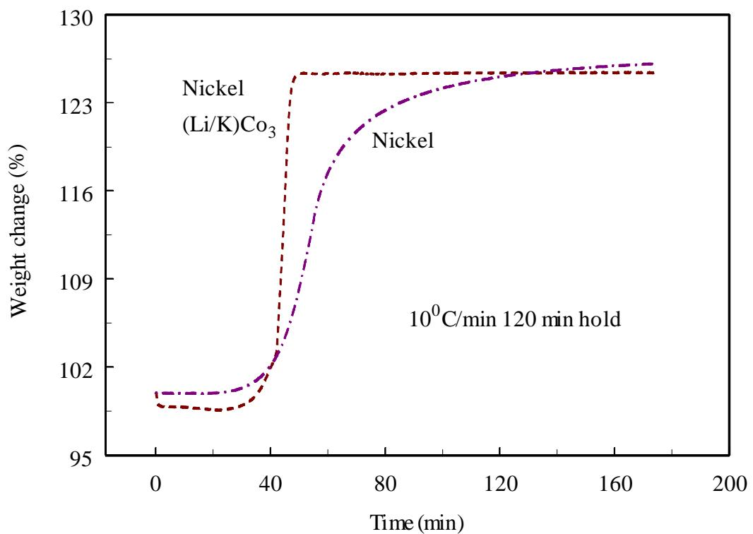
Figure 8a. TGA analysis of sintered nickel tape under cathode gas conditions in the presence and absence of molten carbonate melt.
