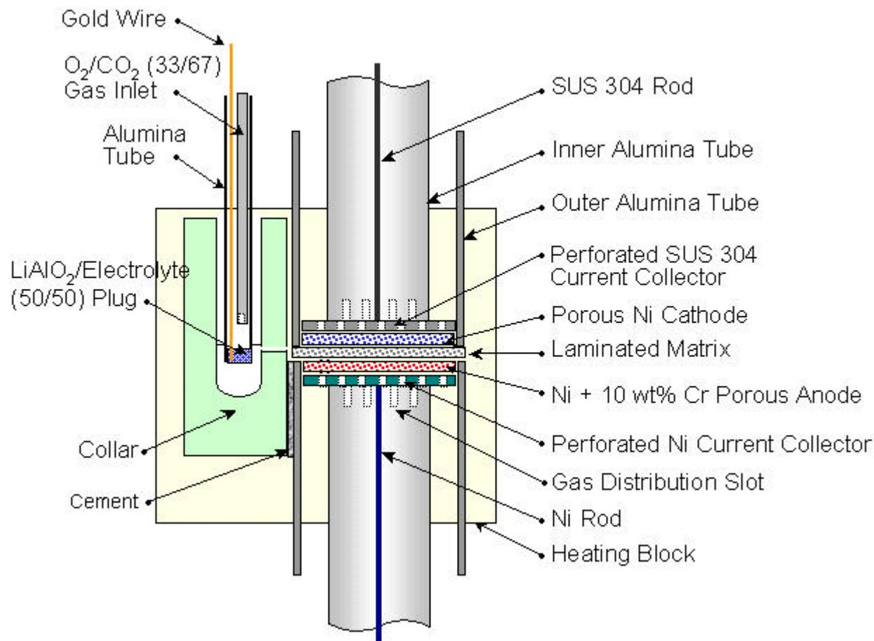
Figure 2b. Schematic diagram of a 3-cm<sup>2</sup>-electrochemical fuel cell. Au/(2CO<sub>2</sub>+1O<sub>2</sub>) reference electrode with a salt bridge was used for measuring cathode and anode potential during polarization studies.
