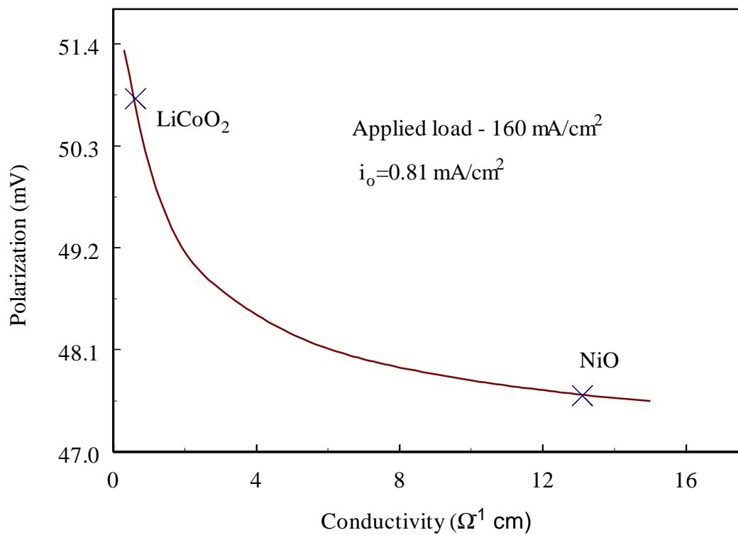
Figure 4. Change in cathode polarization as a function of electrode conductivity. We assume an exchange current density of  $0.81 \text{ mA/cm}^2$  and an applied load of  $160 \text{ mA/cm}^2$ .
