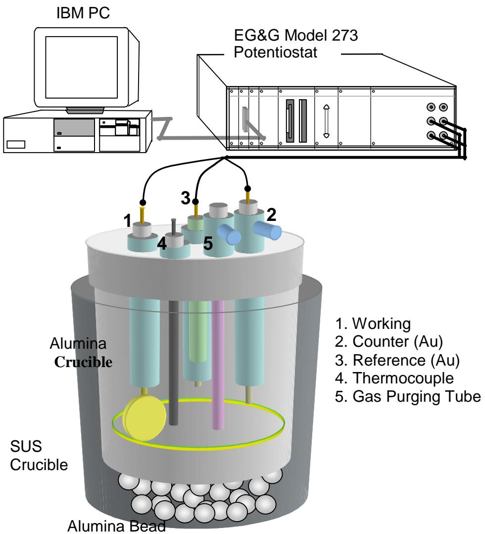
Figure 2a. Schematic diagram of a three-electrode half-cell used for carrying out electrochemical characterization and cathode dissolution studies.
