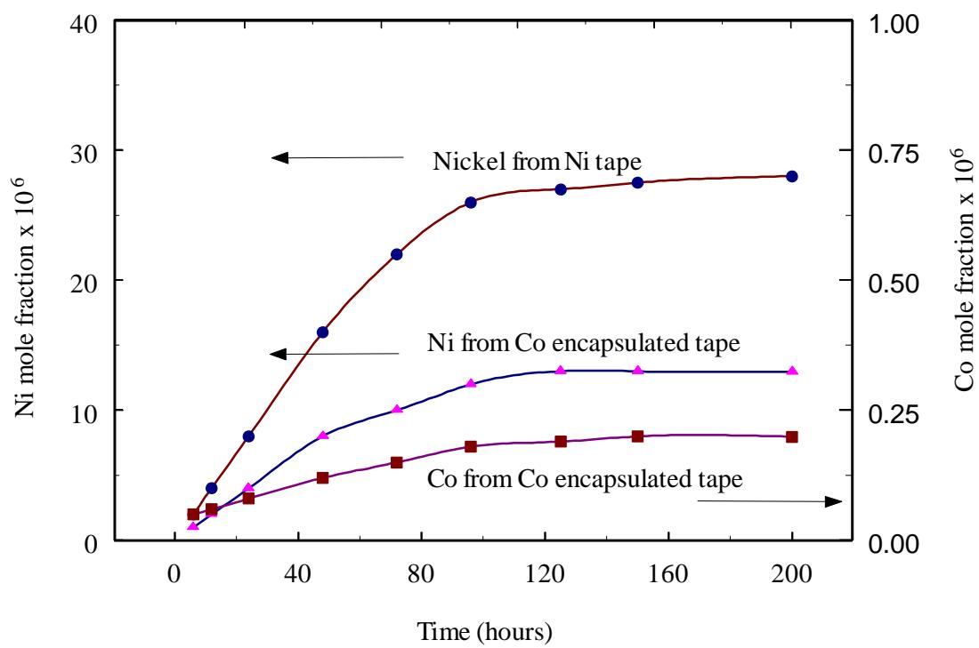
Figure 7. Atomic absorption spectroscopy analysis of dissolved nickel and cobalt in molten carbonate melt.
