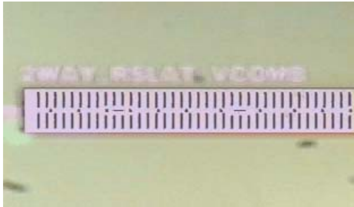
Figure 14. SUMMiT™ Rotational Programmable Grating.
