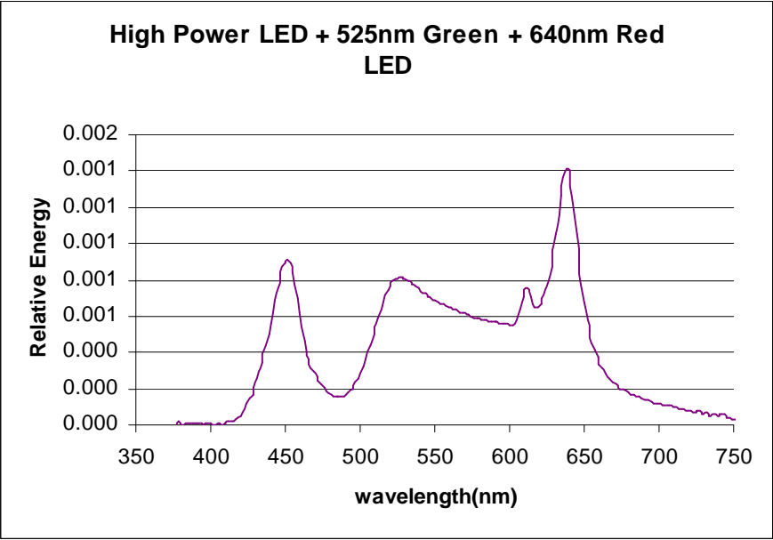
Fig. 22. High Power LED blend with 525nm Green LED and 640nm Red LED
