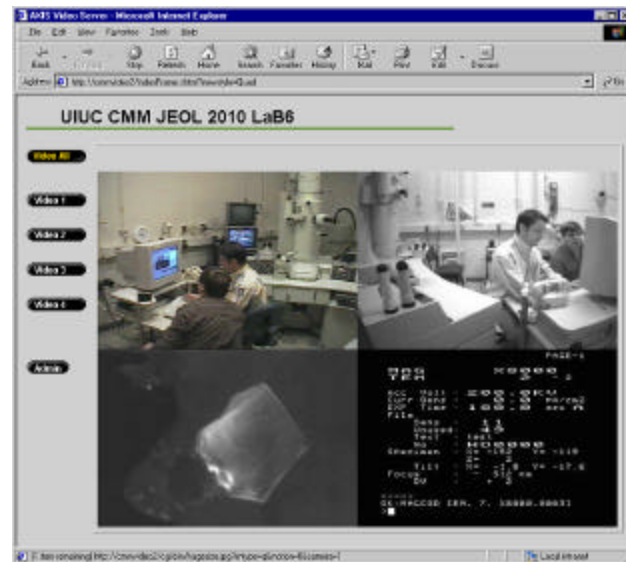
Figure 11 Observe mode browser window for JEOL 2010 TEM. Four video streams including a remote controlled pan-tilt-zoom camera, an infrared camera (room is often darkened for operation), the microscope image, and instrument status screen are provided.
