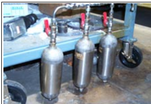
Figure 4 - Liquid Collection System with Hoke Cylinders and Quick Disconnect Valves
