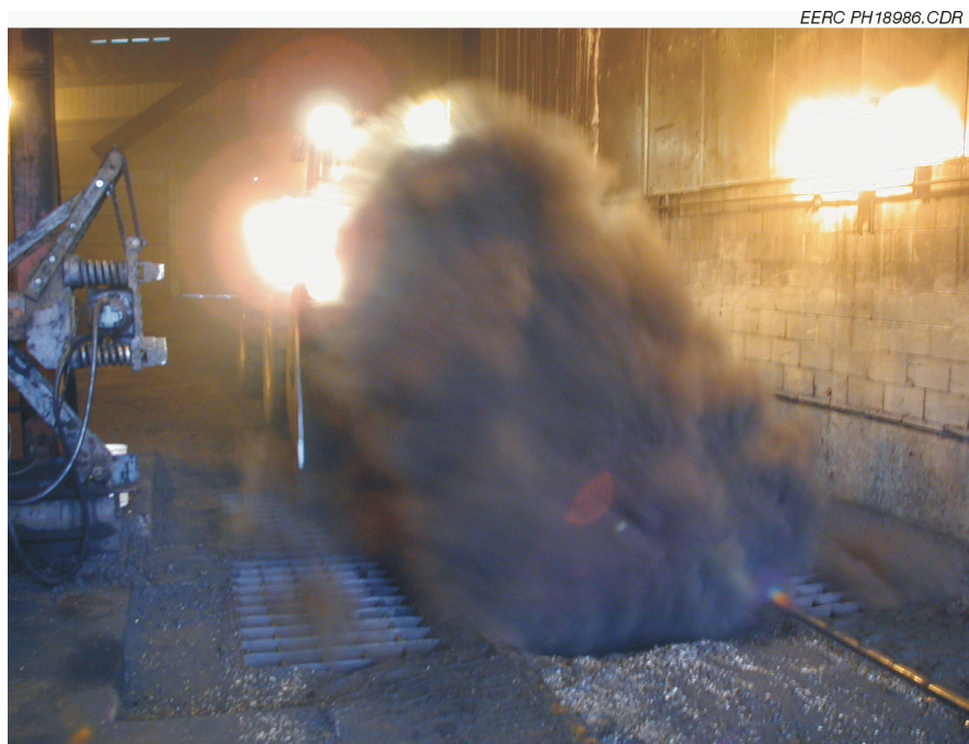
Figure 6. Example of loading fuel into the system and potential dust issues.
