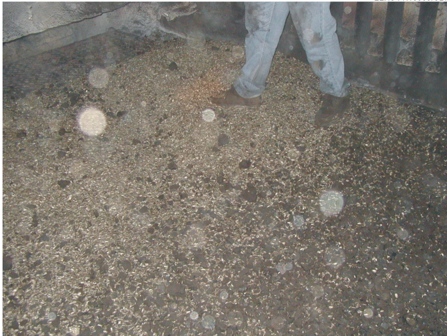
Figure 4. Cold test, Boiler No. 3 – Hulls at stoker end of grate, coal at opposite end.
