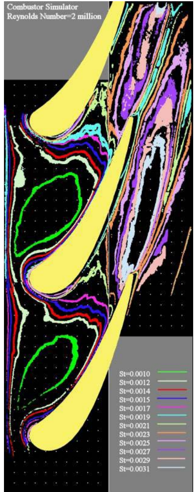
Figure 14. Endwall Stanton number contours, AC, Tu = 0.134 , Lu = 7.3 cm, Re_C = 2,000,000
