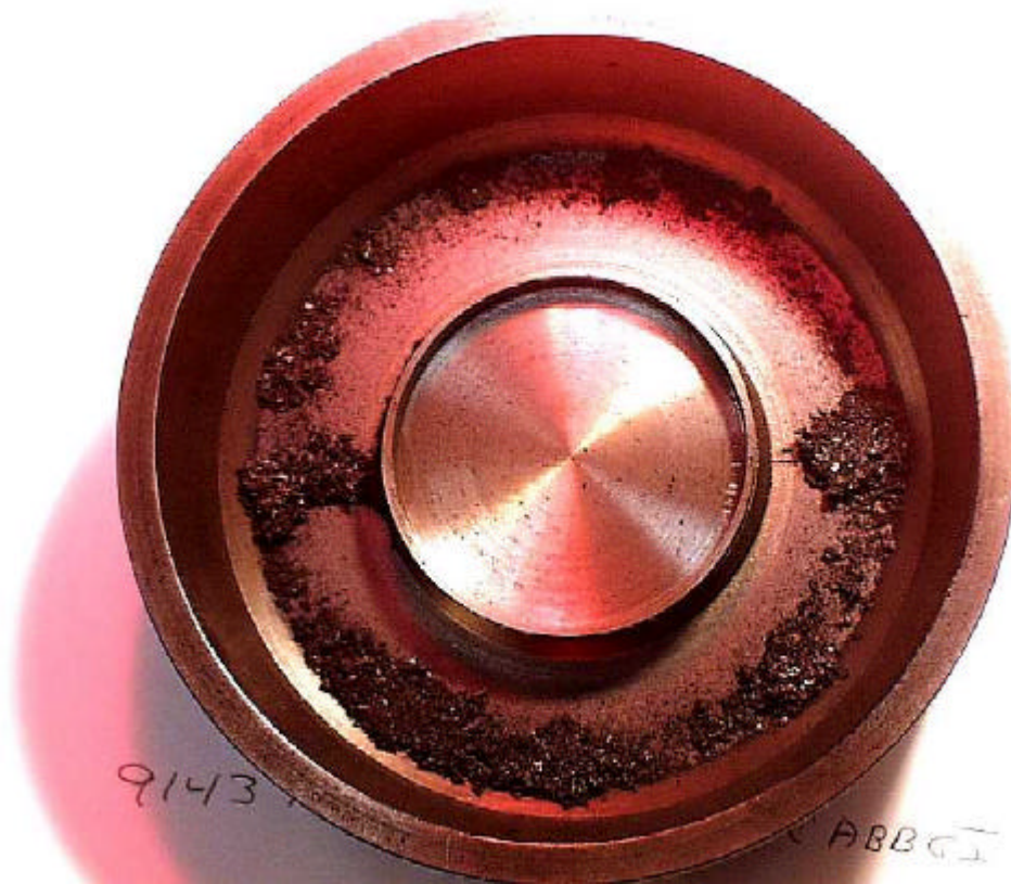
Figure 5-4. AGI Bowl with Pasted Material from Pet Coke/Plastic Pellets
