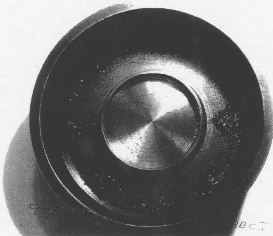
Figure 3 – AGI Bowl with Pasted Material from Pet Coke/Plastic Pellets
