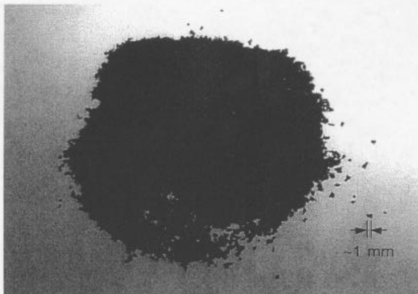
Figure 2 - 80% Pet Coke / 20% Plastic Pellet Prepared to 16 x30 mesh
