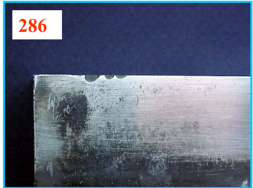
Figure 21: Dissolution at the Corners of Nickel Superalloys 2x2x7 Specimens After 15,000 Cycles
