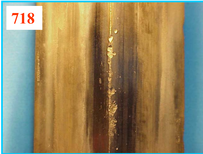
Figure 21: Dissolution at the Corners of Nickel Superalloys 2x2x7 Specimens After 15,000 Cycles
