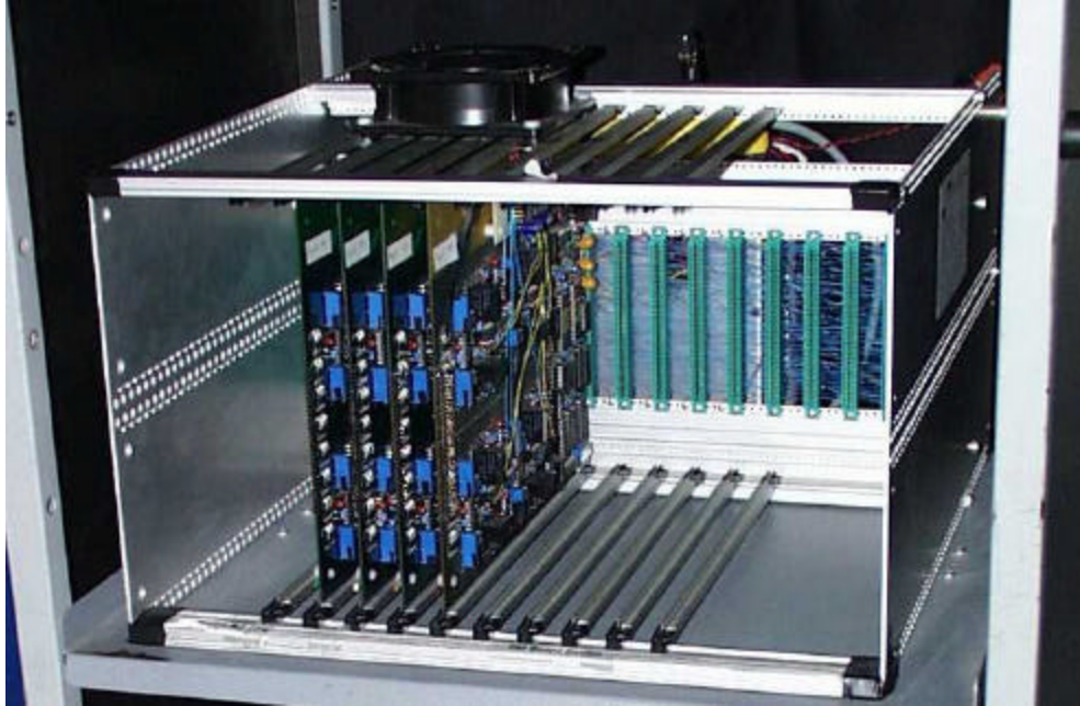
Figure 4.2 Data acquisition computer for Dartmouth EIT imaging system ( www-nml.dartmouth.edu/biomedprg/EIS/index.html ).
