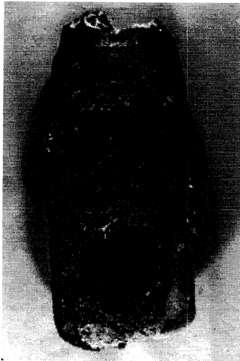
Figure 4. Photograph of the same nozzle sample showing corrosion of powder line and slag coating of refractory surface.
