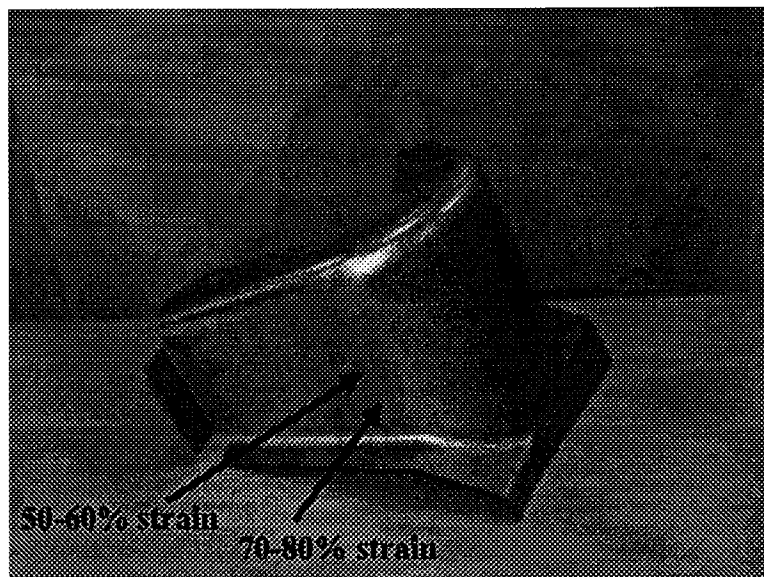
Figure 8. Shock tower part showing regions with major strains of 50-60% and 70-80%
