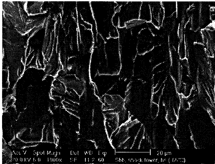
b) Fracture surface in an area with 70-80% strain, specimen fractured at -65°C
