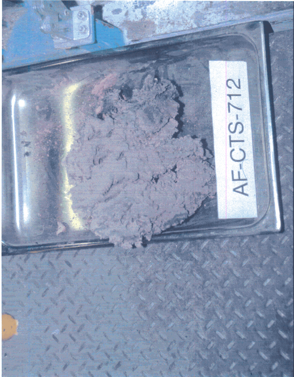
Figure 3.18 Sample of ash deposit collected during a test run at 834,330 Btu/hr
