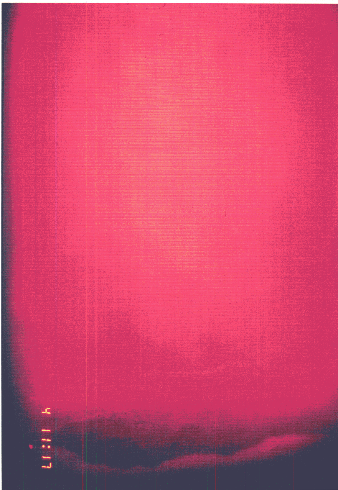
Figure 4.19 Flame at a firing rate of 508,215 Btu/hr adjusted to 0.55 swirl number
