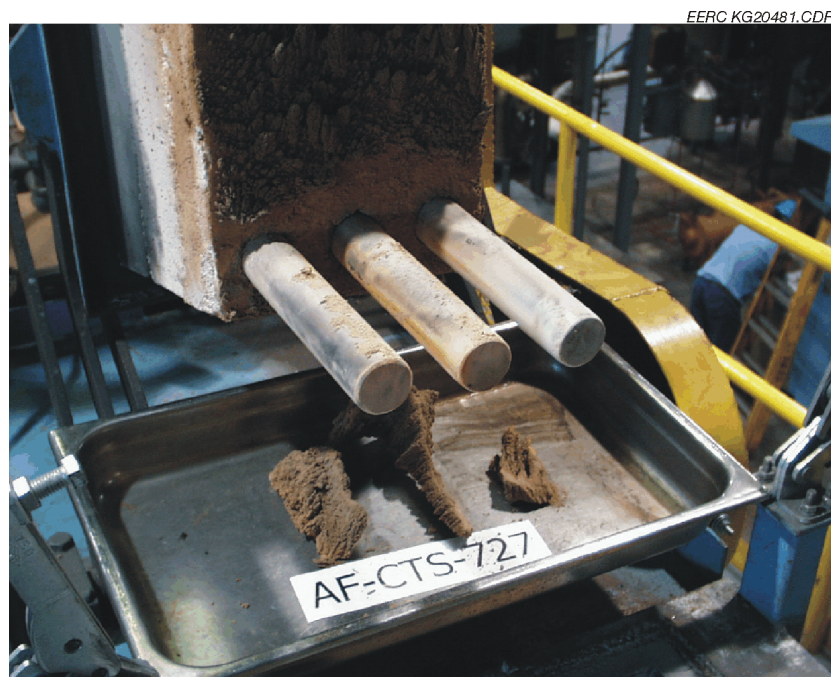
Figure 21. Photograph of the deposit produced by burning Colbert coal–lignin (95:5) blend at a FEGT of 2200°F (1200°C).
