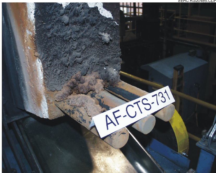
Figure 26. Photograph of the deposit produced by burning a Pittsburgh No. 8 coal at a FEGT of 2350°F (1290°C).
