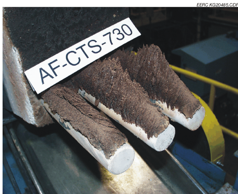
Figure 25. Photograph of the deposit produced by burning a Colbert coal–biosolid (90:10) blend at a FEGT of 2200°F (1200°C).
