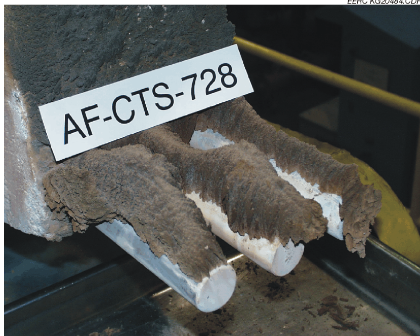
Figure 24. Photograph of the deposit produced by burning a Colbert coal–lignin–biosolid (90:5:5) blend at a FEGT of 2200°F (1200°C).
