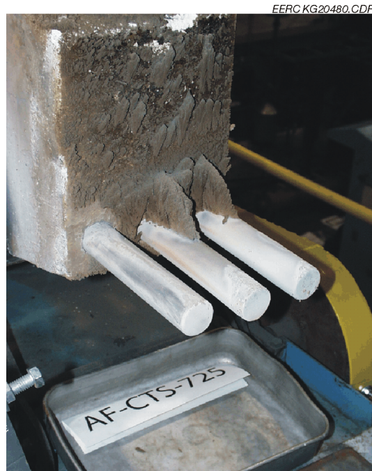
Figure 20. Photograph of the deposit produced by burning Colbert coal at a FEGT of 2200°F (1200°C).
