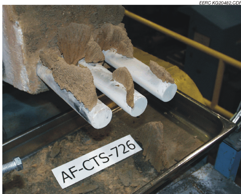
Figure 22. Photograph of the deposit produced by burning a Colbert coal–lignin (90:10) blend at a FEGT of 2200°F (1200°C).
