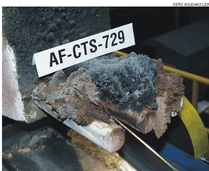
Figure 23. Photograph of the deposit produced by burning Colbert coal–lignin (90:10) blend at a FEGT of 2350°F (1290°C).
