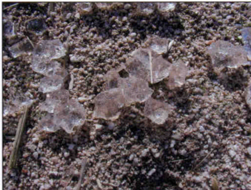
Figure 3-12. Water-insoluble polymer after absorbing water and expanding.
