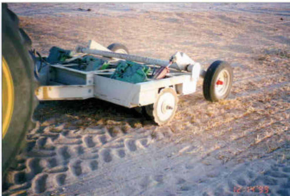
Figure 3-28. The crimper presses straw into the soil orienting the stems vertically.
