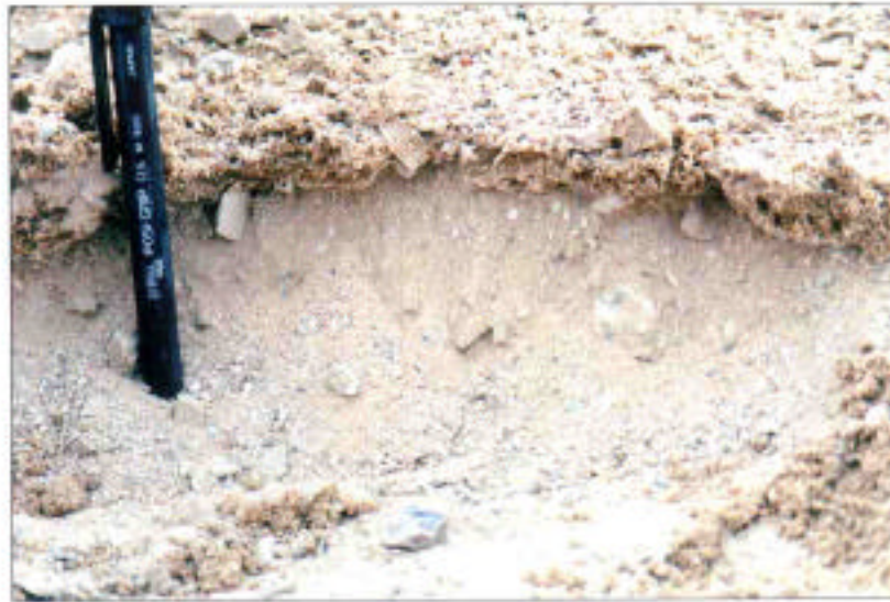
Figure 5-1. Soil crust developed from chemical soil stabilizer that was applied to severely disturbed and highly erodible soils at Fort Irwin, California.
