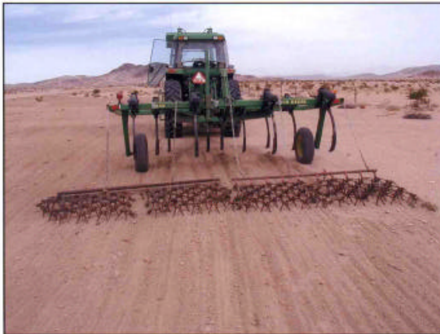
Figure 3-9. Chisel-tooth plow followed by a drag harrow used to reduce compaction and roughen the upper 10-15 cm (4-6 in) of the soil.
