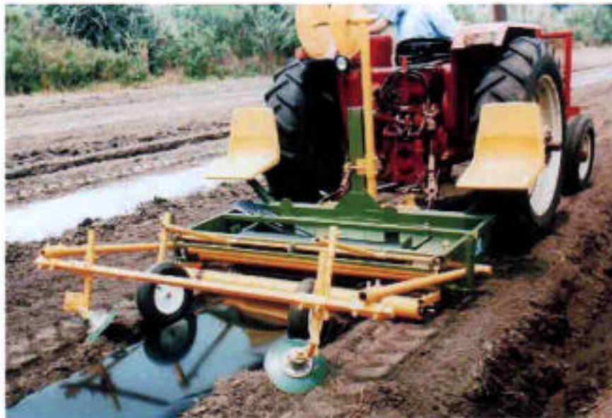
Figure 3-30. Equipment to apply plastic mulch developed for agricultural use could be adapted for use in arid land revegetation.
