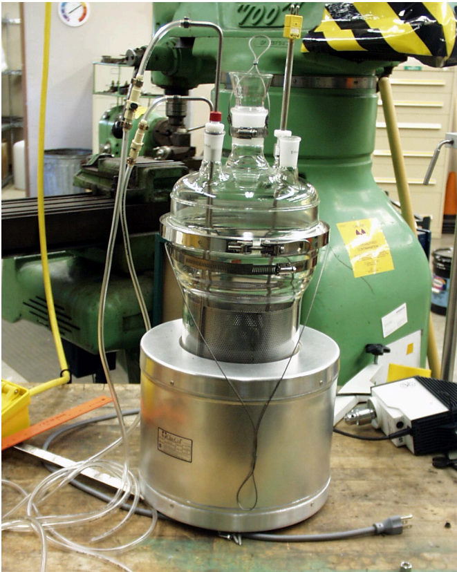
Figure 3. Dissolver with heating mantle on benchtop in mock-up laboratory before introduction to remote cell.
