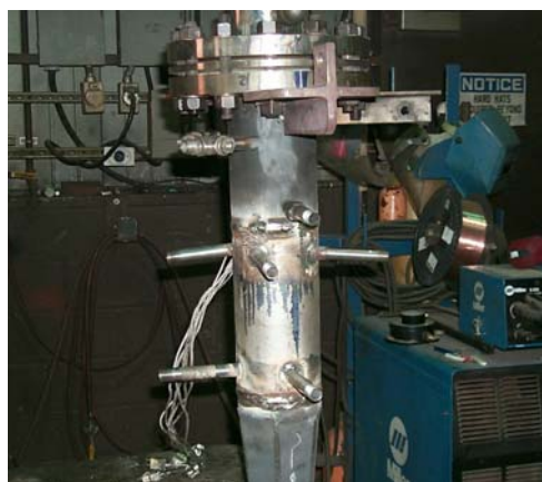
Figure 2. Modified gas-fired combustor for pilot-scale testing
