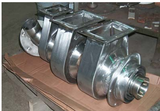
Figure 4. Original PC burner used for pilot-scale PC Preheat testing
