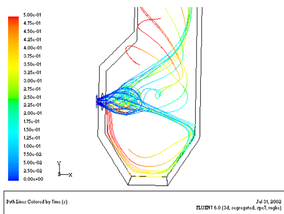
Figure 9. Fuel particle path lines with the original PC burner design
