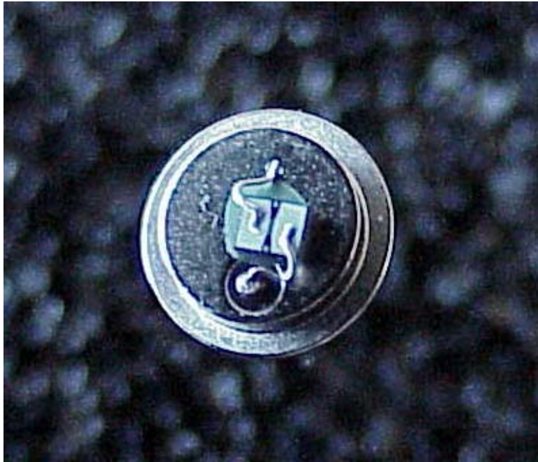
Figure 2- 6. TO46 Header with 3-2B1 SCB Mounted in Perpendicular Orientation.
