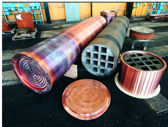
Figure 28.11. Copper canister with nodular cast-iron insert for BWR fuel
