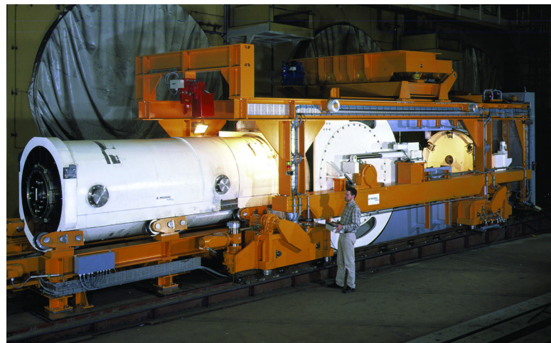
Figure 28.7. SKB has developed a prototype of a remote-controlled and radiation-shielded deposition machine
