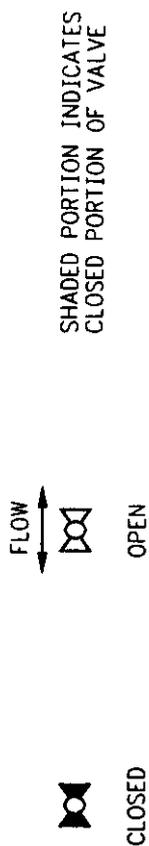
FIGURE 1. VALVE POSITION CONFIGURATIONS
