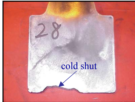
Rating = 2 Significant cold shuts
