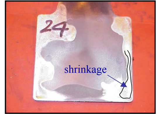
Rating = 4 Significant shrinkage
