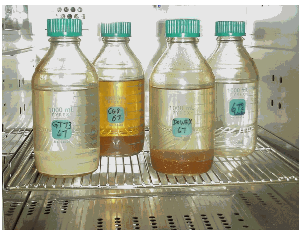
Figure 1. Experimental Setup at 70° C with GT73, CG8, and Dowex21K Resins and a Control with Water Only.
