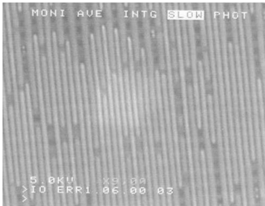
Figure 4.16 – Two-layer 0.4 micron epoxy sample made on 2-12-2001 with the higher viscosity epoxy. Epoxy applied 4, 4, 4, 4, and 4 times before another epoxy mixture was made and then 4, 4, and 4 times more. Furnace times of 5 minutes again.
