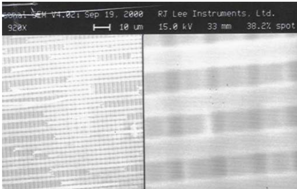
Figure 4.5 – Two-layer 2.5 micron epoxy sample made on 9-15-2000. Epoxy was applied with sweeps of 6, 6, and 6 times with 5-10 minutes in the furnace between applications.
