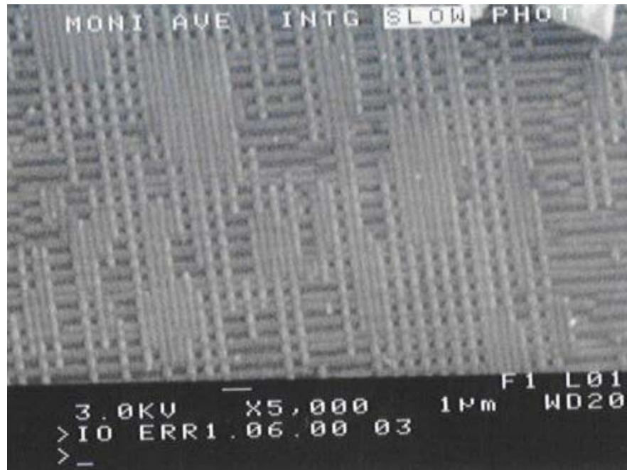
Figure 4.15 – Attempted two-layer 0.4 micron epoxy sample made on 2-6-2001. Epoxy applied 3.5 and 2.5 then mixed then 3.5 and 2.5 then mixed then 3.5 times across. Furnace times of 5 minutes in between applications.
