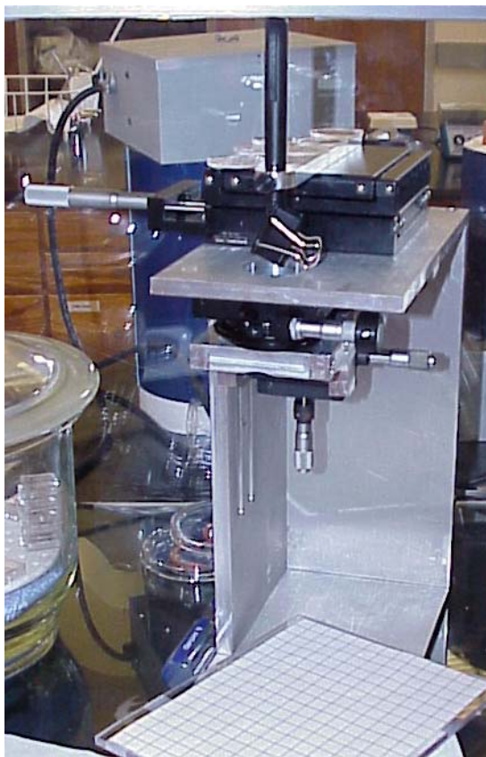
Figure 4.2 – Laser alignment system designed for the 2.5 and 1.0 \mu\text{m} samples
