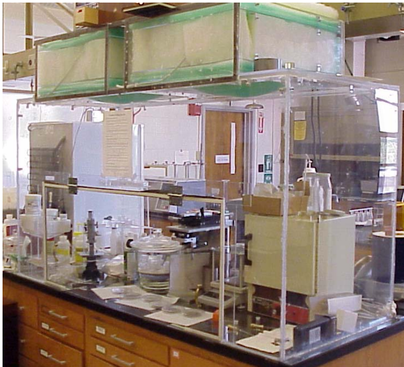
Figure 4.1 – Clean box built to house the fabrication process of epoxy molds
