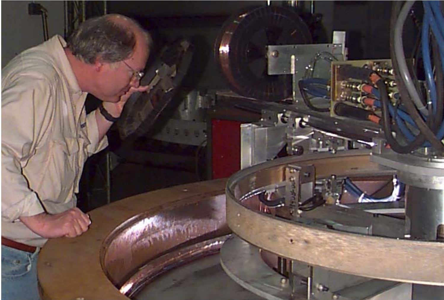
Fig. 1. Photograph of semiautomatic rotary remote welding system
