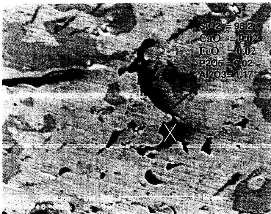
Figure 19: SEM micrograph of polished Midrex HBI cross section. The approximate chemical composition of the indicated oxide feature was measured via EDS.
