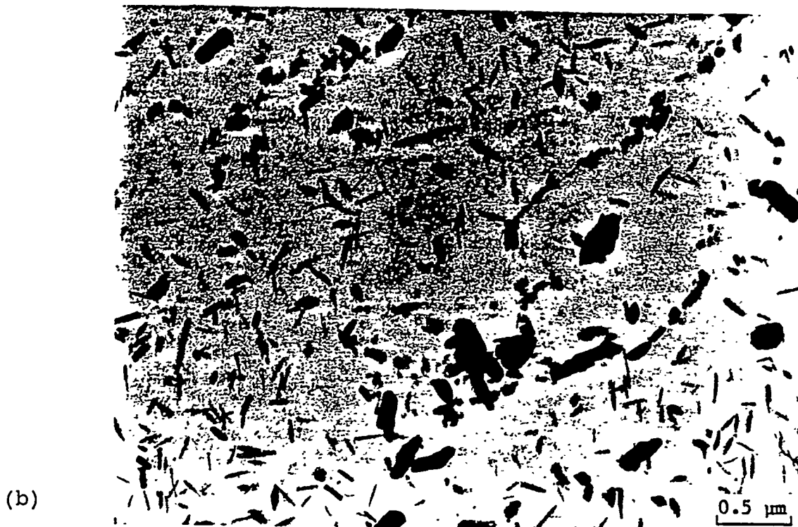
Figure 5. Extraction replicas of 3Cr-1.5MoV steel (a) after quenching and tempering 8 h at 663°C and (b) after normalizing and tempering 8 h at 663°C.
