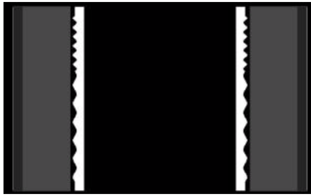
Figure 2. The Rus-6 simulated geometry through the center of the load without projection. Black= vacuum. White = copper test object with sinusoidal surface. Moving outward, dark gray = polyethylene, even darker gray = aluminum liner.
