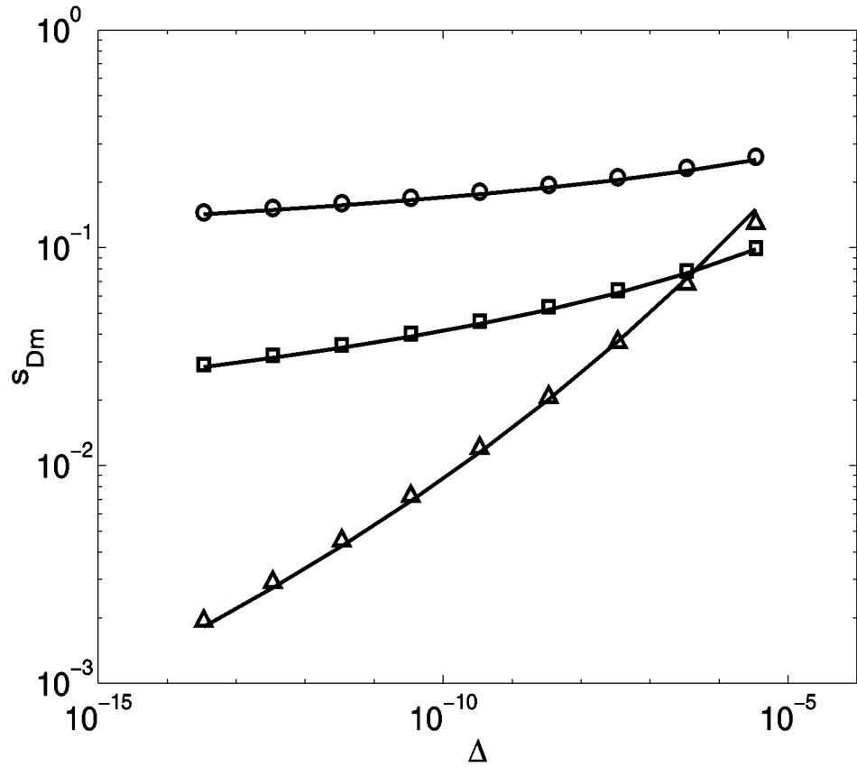
Figure 7: Maximum rescaled supersaturation,  $s_{Dm}$ , as a function of  $\Delta$  for various cavity size distributions. Solid lines correspond to the simpler problem, points correspond to the full numerical solution [denoted by circles for the Rayleigh cavity size distribution, by triangles for a stretched exponential ( $n = 0.2233$  and  $\sigma = 0.1364$ ) and by squares for a stretched exponential ( $n = 1.0$  and  $\sigma = 1.0$ )].
