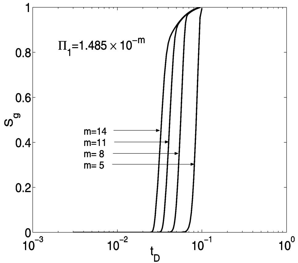
Figure 4: Variation of the gas saturation,  $S_g$ , as a function of dimensionless time,  $t_D$ . Effect of  $\Pi_1 = 1.485 \times 10^{-m}$ , for  $\Pi_2 = 9.6972 \times 10^7$ ,  $\Pi_\rho = 2.981$ ,  $\Pi_c = 0.117 \times 10^1$  and  $\Pi_H = 0$ .
