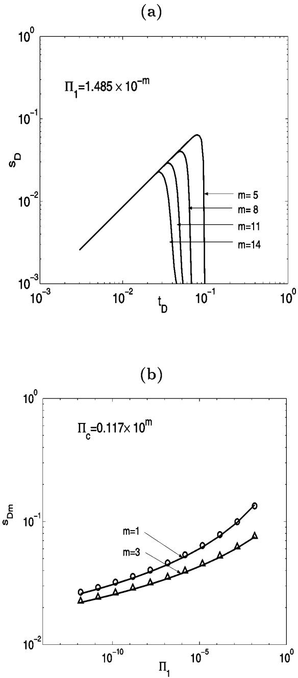
Figure 3: Numerical results for the rescaled supersaturation,  $s_D$ : (a) Variation as a function of dimensionless time,  $t_D$ . Effect of  $\Pi_1 = 1.485 \times 10^{-m}$ , for  $\Pi_2 = 9.6972 \times 10^7$ ,  $\Pi_\rho = 2.981$  and  $\Pi_H = 0$ . (b) Effect of the parameter  $\Pi_1$  on the maximum rescaled supersaturation,  $s_{Dm}$ , for  $\Pi_c = 0.117 \times 10^m$ . Points correspond to the full numerical solution, solid lines correspond to the simpler problem.
