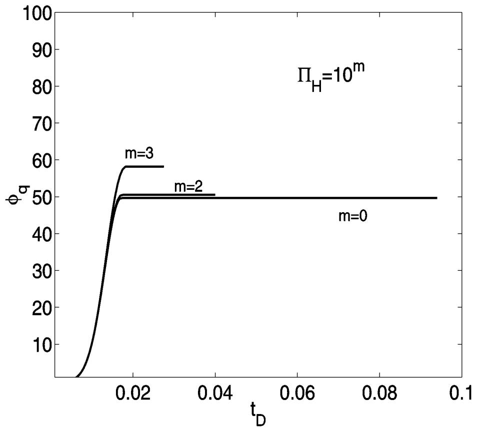
Figure 5: Variation of the rescaled nucleation fraction,  $\phi_q$ , as a function of dimensionless time,  $t_D$ . Effect of  $\Pi_H = 10^m$ , for  $\Pi_1 = 1.485 \times 10^{-8}$ ,  $\Pi_2 = 9.6972 \times 10^7$ ,  $\Pi_c = 0.117 \times 10^1$  and  $\Pi_\rho = 2.981$ .
