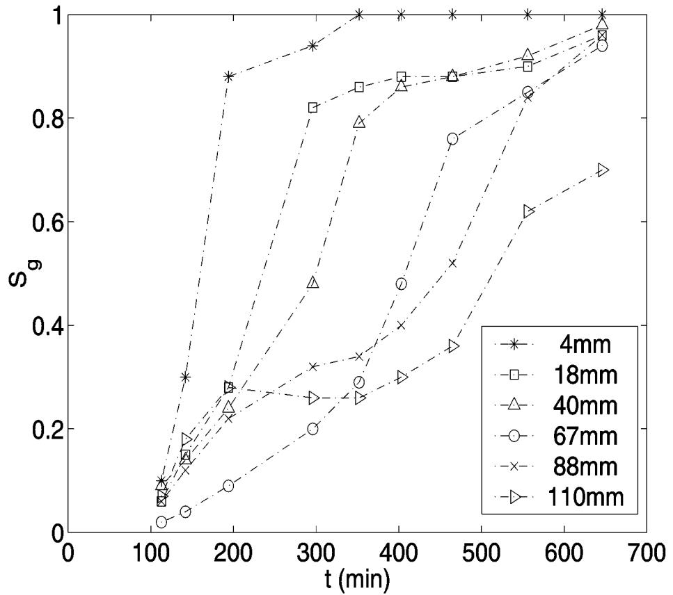
Figure 8: Gas saturation profiles for single-phase flash experiment as a function of time and for various axial positions along the core,  $L$ . Experimental data from Dehghani et al., (1997).
