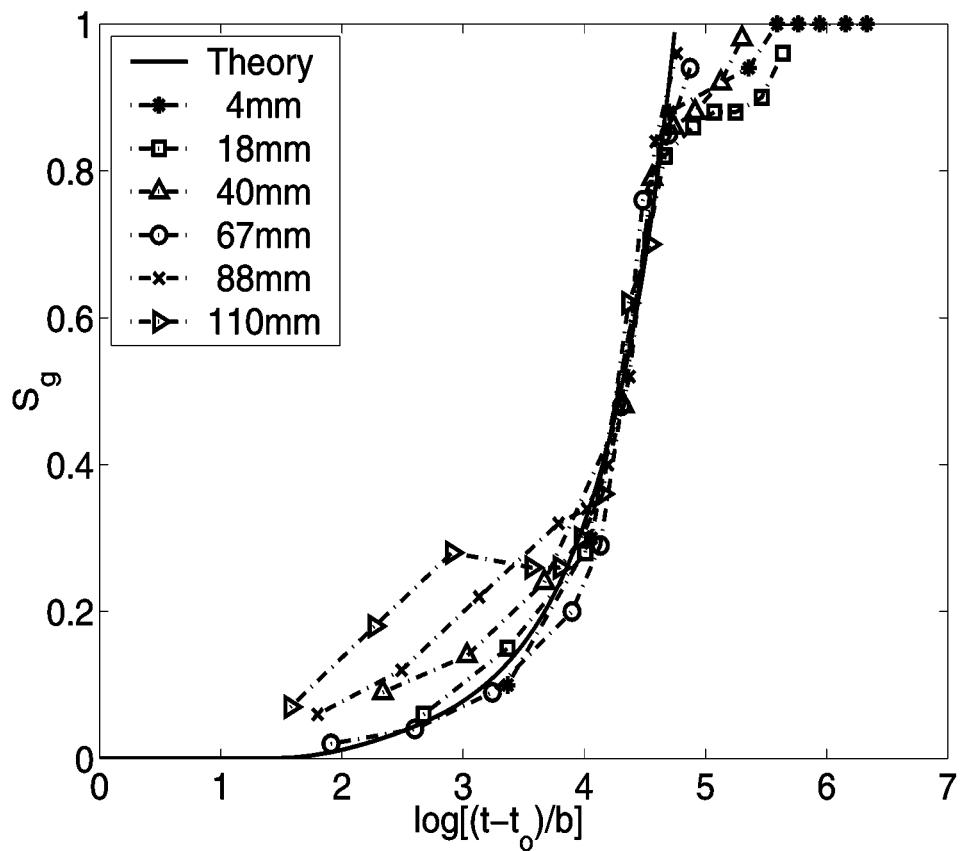
Figure 9: The evolution of the gas saturation as a function of a rescaled time for the experiments of Dehghani et al., (1997). Points denote experimental values and the solid line corresponds to the full numerical solution.
