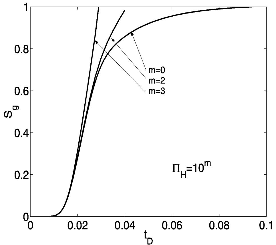
Figure 6: Variation of the gas saturation,  $S_g$ , as a function of dimensionless time,  $t_D$ . Effect of  $\Pi_H = 10^m$ , for  $\Pi_1 = 1.485 \times 10^{-8}$ ,  $\Pi_2 = 9.6972 \times 10^7$ ,  $\Pi_c = 0.117 \times 10^1$  and  $\Pi_\rho = 2.981$ .
