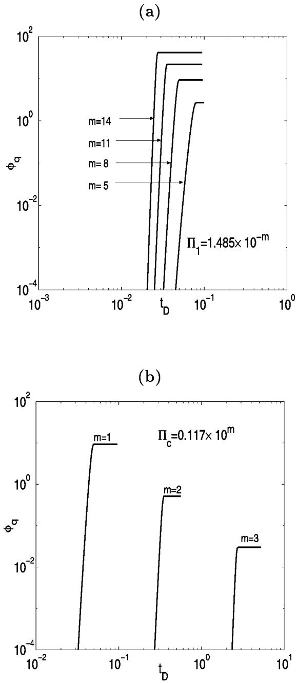
Figure 1: Variation of the rescaled nucleation fraction,  $\phi_q$ , as a function of the dimensionless time,  $t_D$ . (a) Effect of  $\Pi_1 = 1.485 \times 10^{-m}$ , for  $\Pi_2 = 9.6972 \times 10^7$ ,  $\Pi_\rho = 2.981$  and  $\Pi_H = 0$ . (b) Effect of  $\Pi_c = 0.117 \times 10^m$ , for  $\Pi_1 = 1.485 \times 10^{-8}$ ,  $\Pi_2 = 9.6972 \times 10^7$ ,  $\Pi_\rho = 2.981$  and  $\Pi_H = 0$ .
