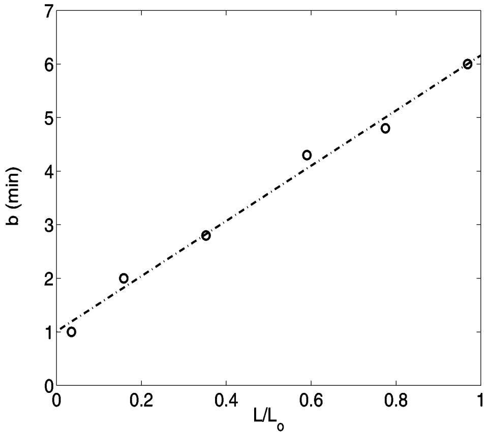
Figure 10: Variation of the rescaling factor,  $b$ , as a function of the dimensionless axial position along the core,  $L/L_o$ .
