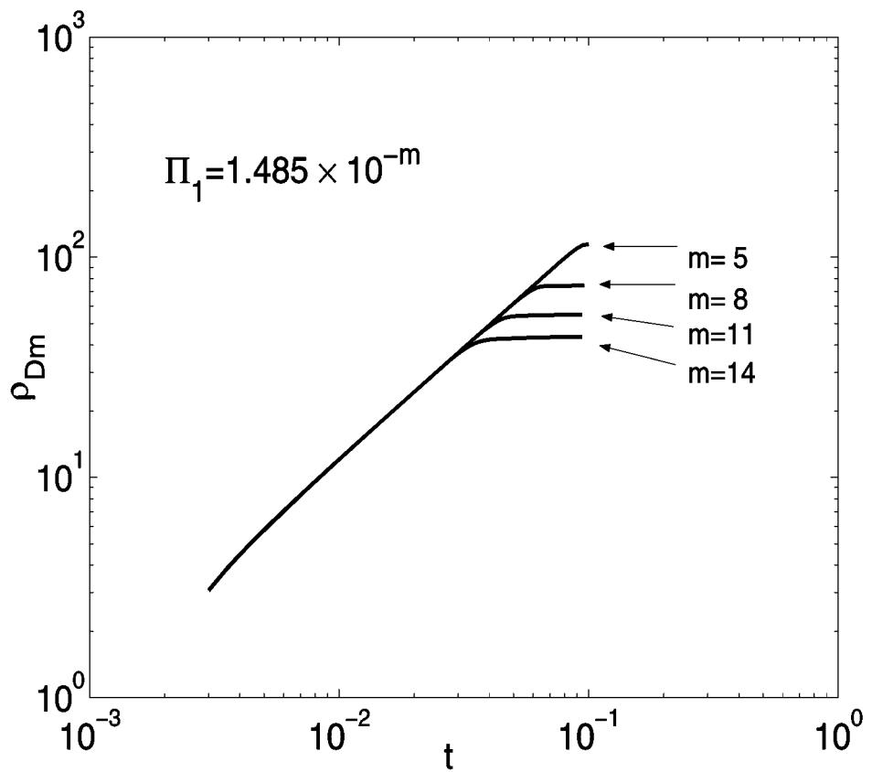
Figure 2: Variation of the mean rescaled dimensionless radius,  $\rho_{Dm}$ , as a function of dimensionless time,  $t_D$ . Effect of  $\Pi_1 = 1.485 \times 10^{-m}$ , for  $\Pi_2 = 9.6972 \times 10^7$ ,  $\Pi_\rho = 2.981$ ,  $\Pi_c = 0.117 \times 10^1$  and  $\Pi_H = 0$ .
