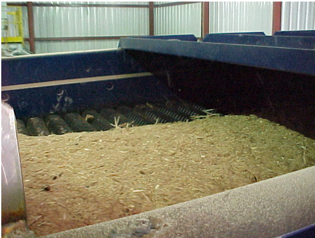
Figure 4-3. Sawdust Being Screened on the Disc Screen
