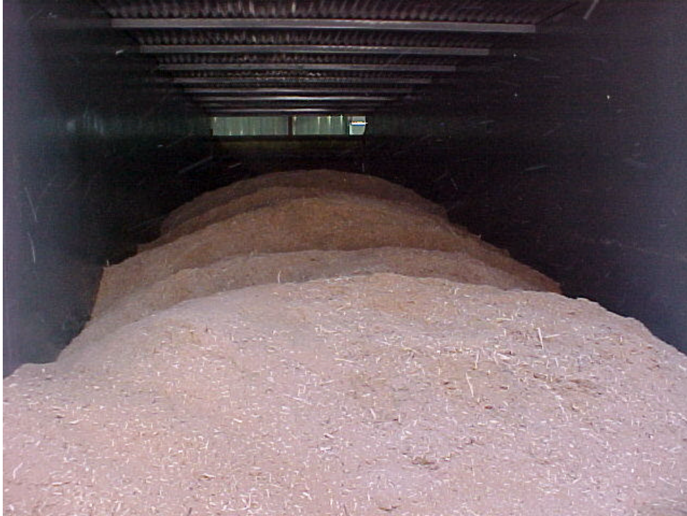
Figure 4-2. Sawdust Being Transported Up the Walking Floor Unloader
