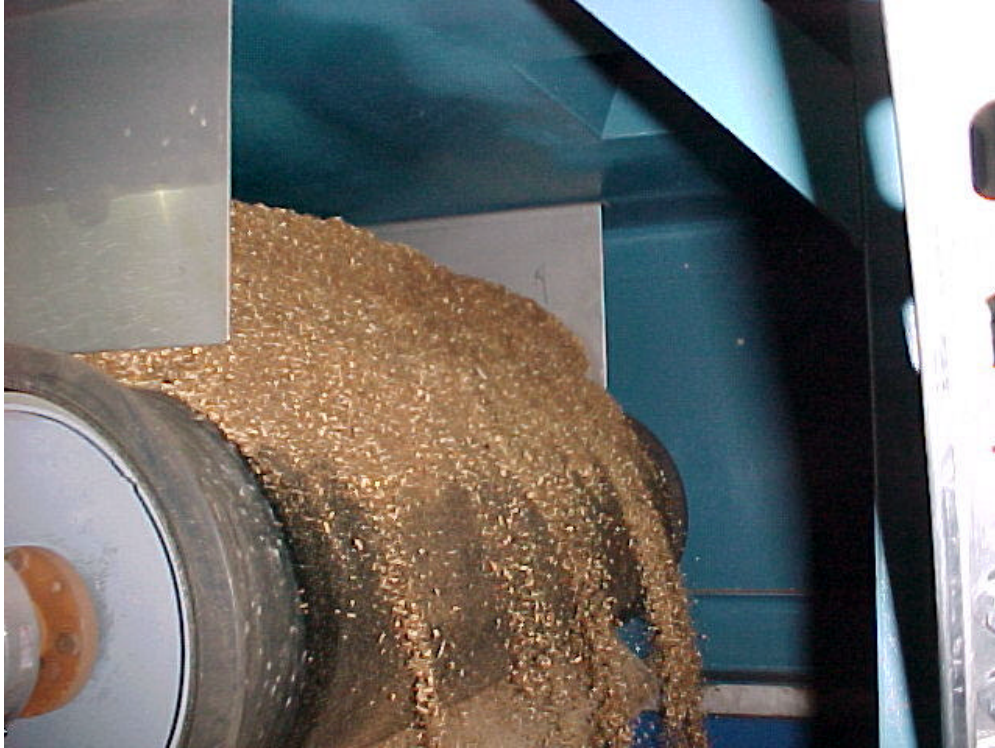
Figure 4-4. Sawdust Being Metered on the Weigh Belt Feeder
