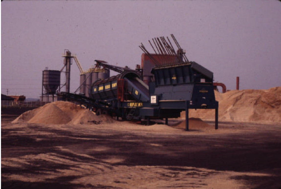
Figure 2-3. The Trommel Screen Installed at the Allen Fossil Plant
