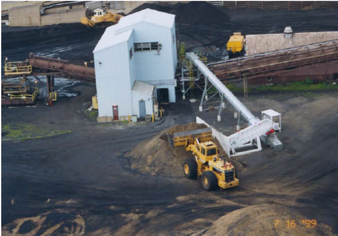
Figure 5-13. The Above Ground Reclaim and Conveyor System Used for Cofiring at Bailly Generating Station
