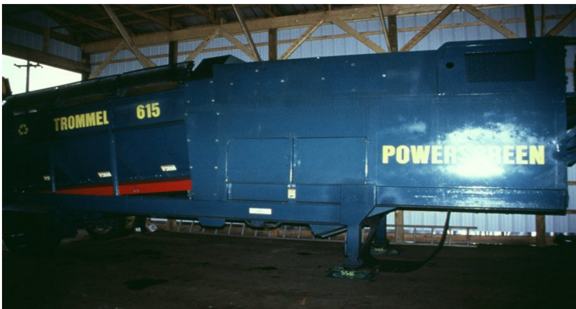
Figure 3-15. Installation of the Trommel Screen for Sawdust Preparation at Seward Generating Station
