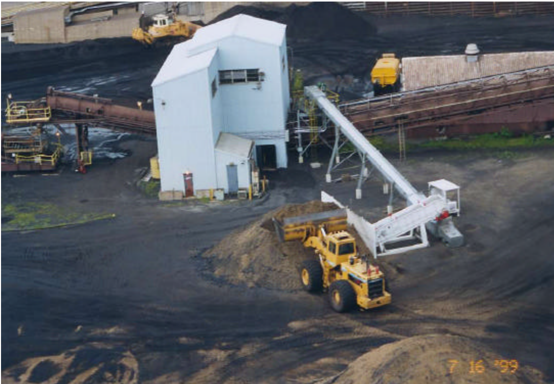
Figure S-17. Operation of the Reclaim and Opportunity Fuel/Coal Blending System at Bailly Generating Station
