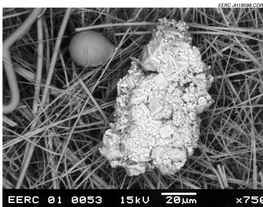
Figure 19. SEM photograph of the surface of the EPA Method 5 particle filter from the test of the 60-ppi combustion SGD.
