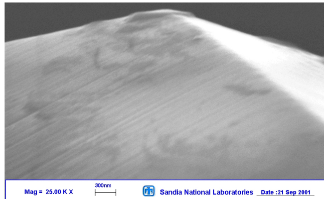
Figure 5.8: A SEM image of the diamond tip used to nanoindent MgO, magnification = 25,000 \times .
