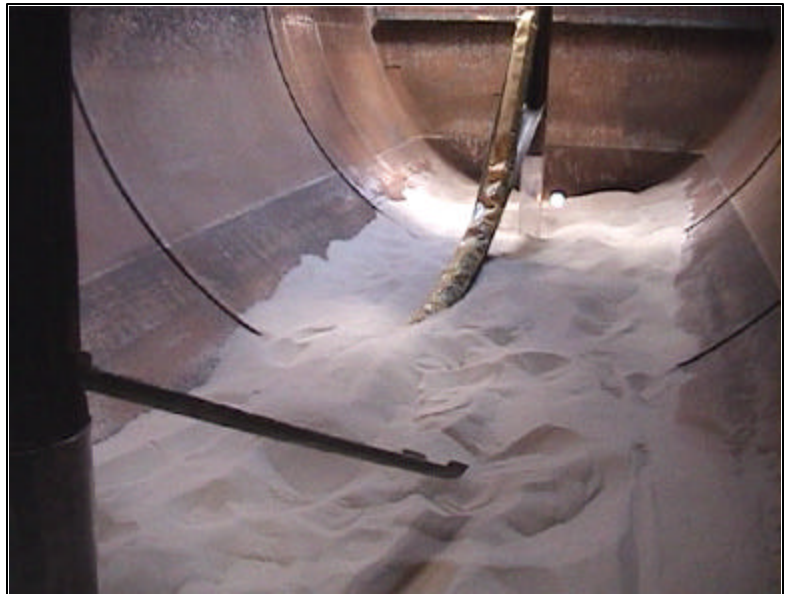
Figure 4. Deployment of horizontal injection tool through sand in Savannah River tank mock-up.
