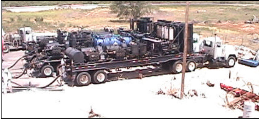
Figure 3. Trailers with high-pressure pumps.
