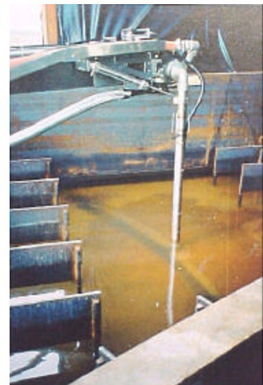
Figure 1. AWRS telescopic arm deployed in a test tank.
