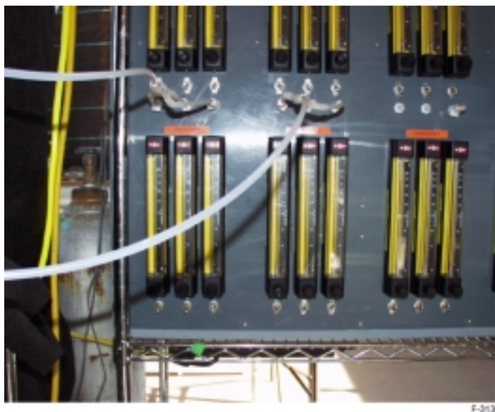
Figure 11. Partial front view of the pH control and gas distribution system showing the rotameters and outlets that distribute the gas mixtures into the chemostats. Each channel controls gas flow through three rotameters. The mix of three different gas streams results in the desired composition to mimic different industrial flue gases.
