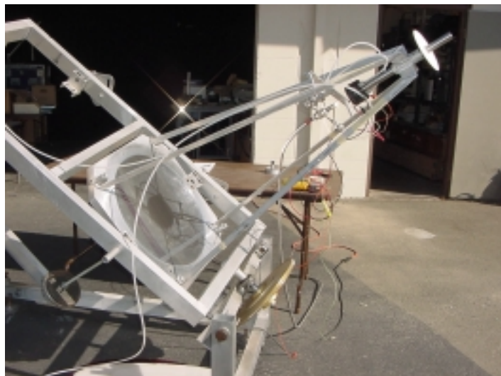
Figure 71. Experimental facility for GaSb cell performance tests with the IR solar spectra.
