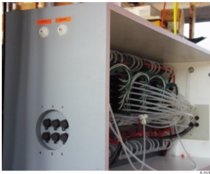
Figure 10. Rear and side view of the pH control and gas distribution system showing two ports (top) to accept gas mixtures for distribution to 12 different channels and 6 ports to accept input from 6 different pH probes. Six more probe ports are found on the opposite side (out of view).
