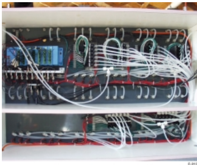
Figure 9. Rear view of the pH control and gas distribution system showing the I/O modules as well as tubes and solenoids that distribute and feed the gas mixtures to the chemostat cultures.
