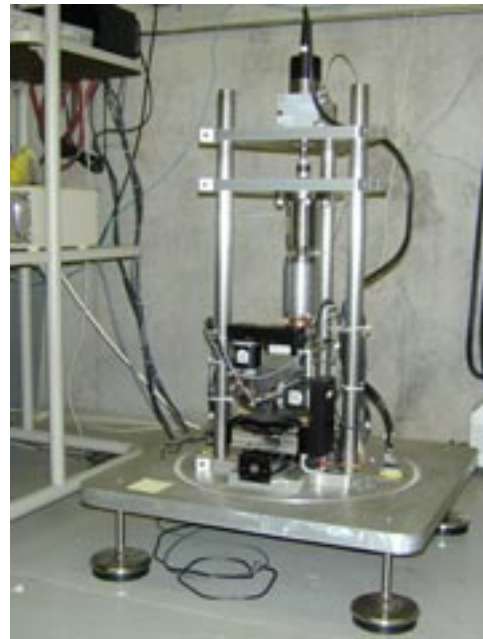
FIGURE 5: Magnetic bearing element test stand
