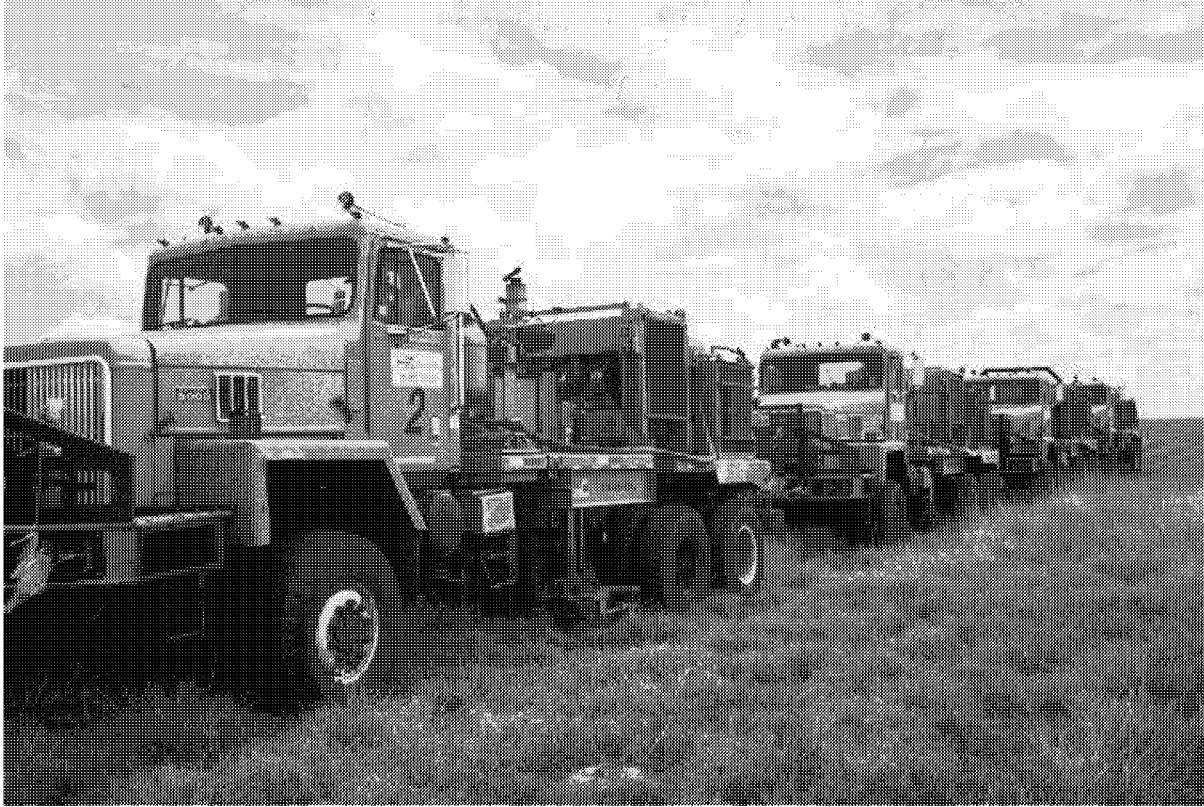
Figure 3.1.3a. Vibroseis trucks lining up to begin the survey at Eva South. These are conventional vibroseis trucks that generate standard P-waves.
