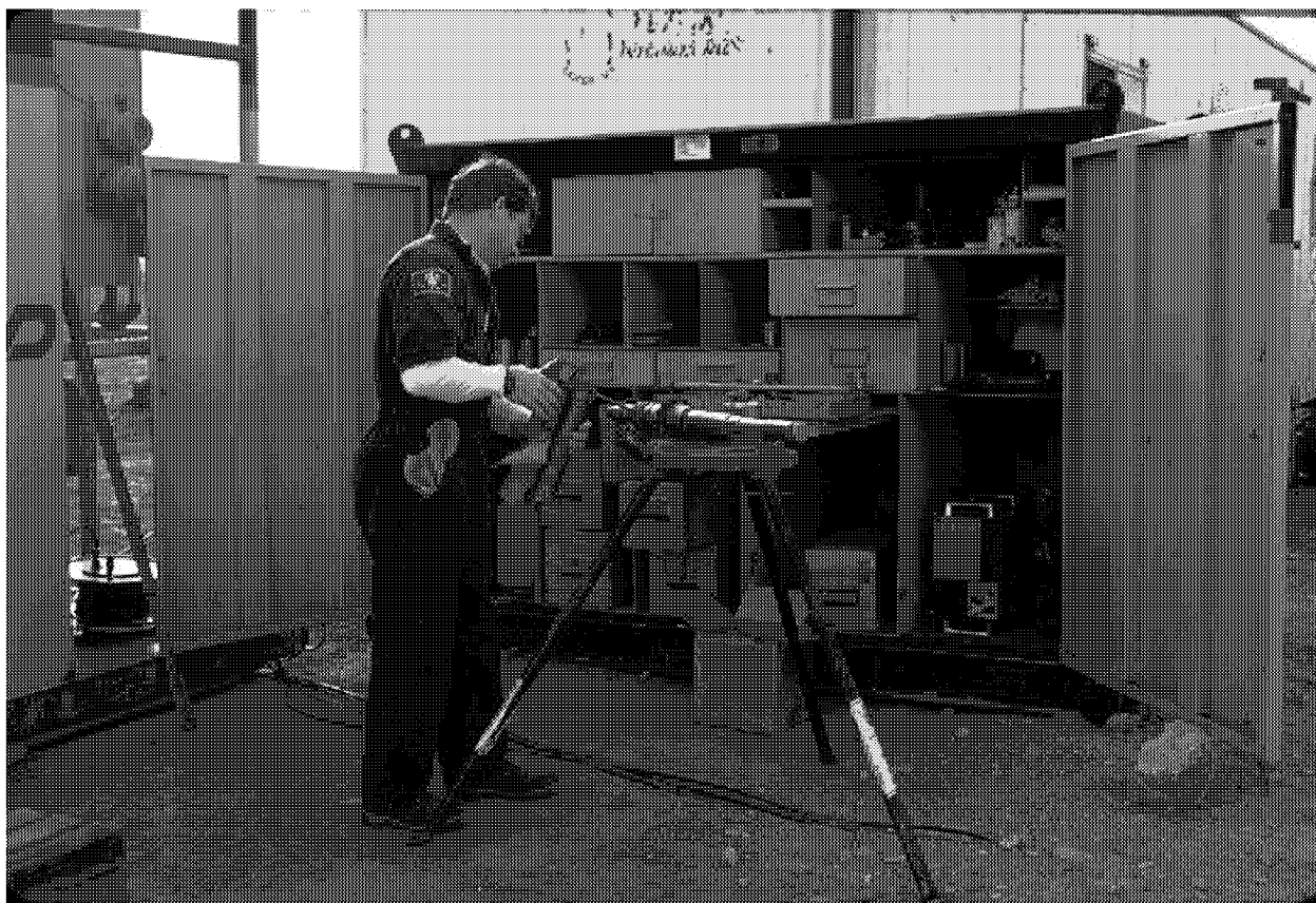
Figure 4.2.1b. Photograph of a technician preparing the MWD (measurement while drilling) tool prior to horizontal drilling. This tool, along with the rest of the drilling assembly and drill pipe became permanently stuck in the hole.
