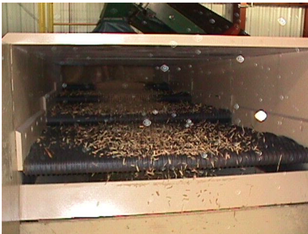
Figure 3. Screening sawdust at the Willow Island Generating Station
