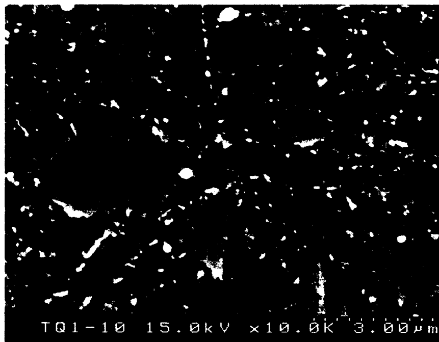
Fig. 12(d) SEM micrograph of TQ1 after 10-hour tempering under 1200°F
