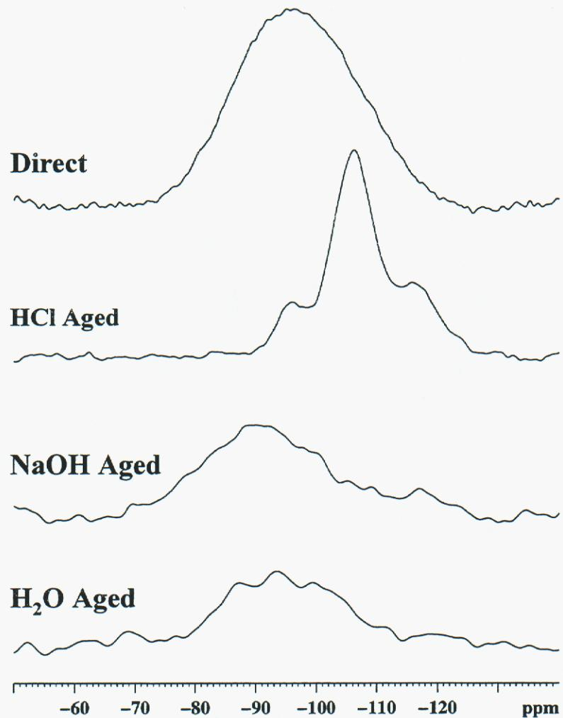
**Figure 23:**  $^{29}\text{Si}$  CPMAS NMR spectra of aged aluminum borosilicate glass.
