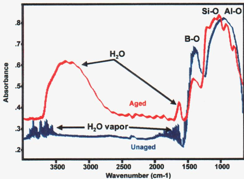
**Figure 15. Infrared transmission spectra of (aged and unaged) bulk aluminum borosilicate glass.**
