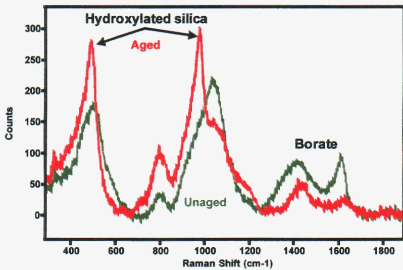
Figure 14. Raman spectra of bulk aluminum borosilicate glass (aged and unaged).
