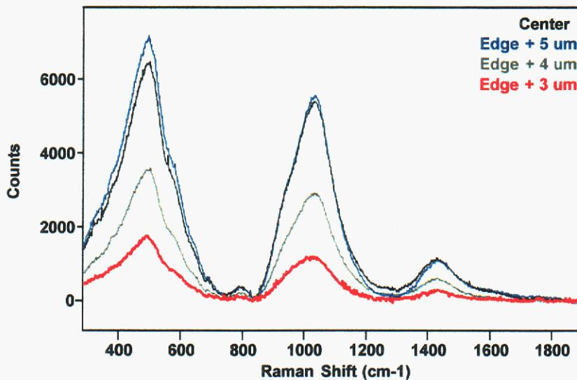
**Figure 19. Micro-Raman spectra of inner locations on the end of the aged fiber (same fiber as Figure 18).**
