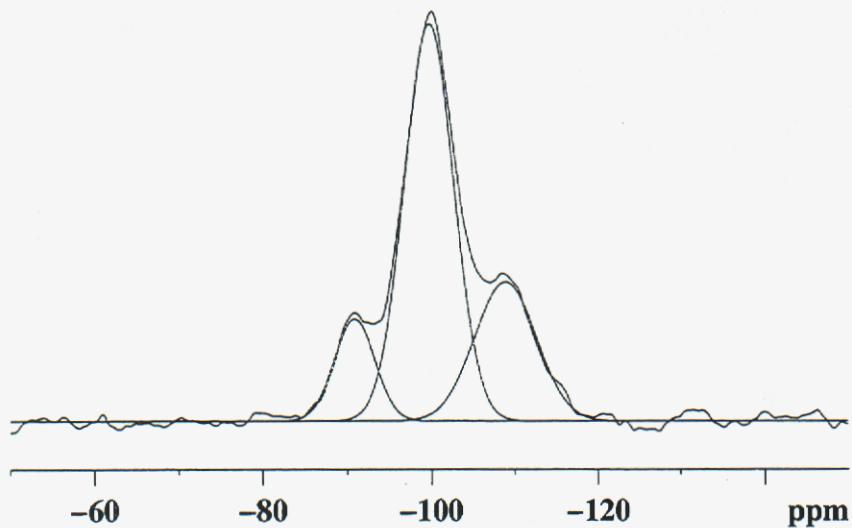
**Figure 22: Deconvolution of  $^{29}\text{Si}$  NMR spectra of acid aged aluminum borosilicate glass.**
