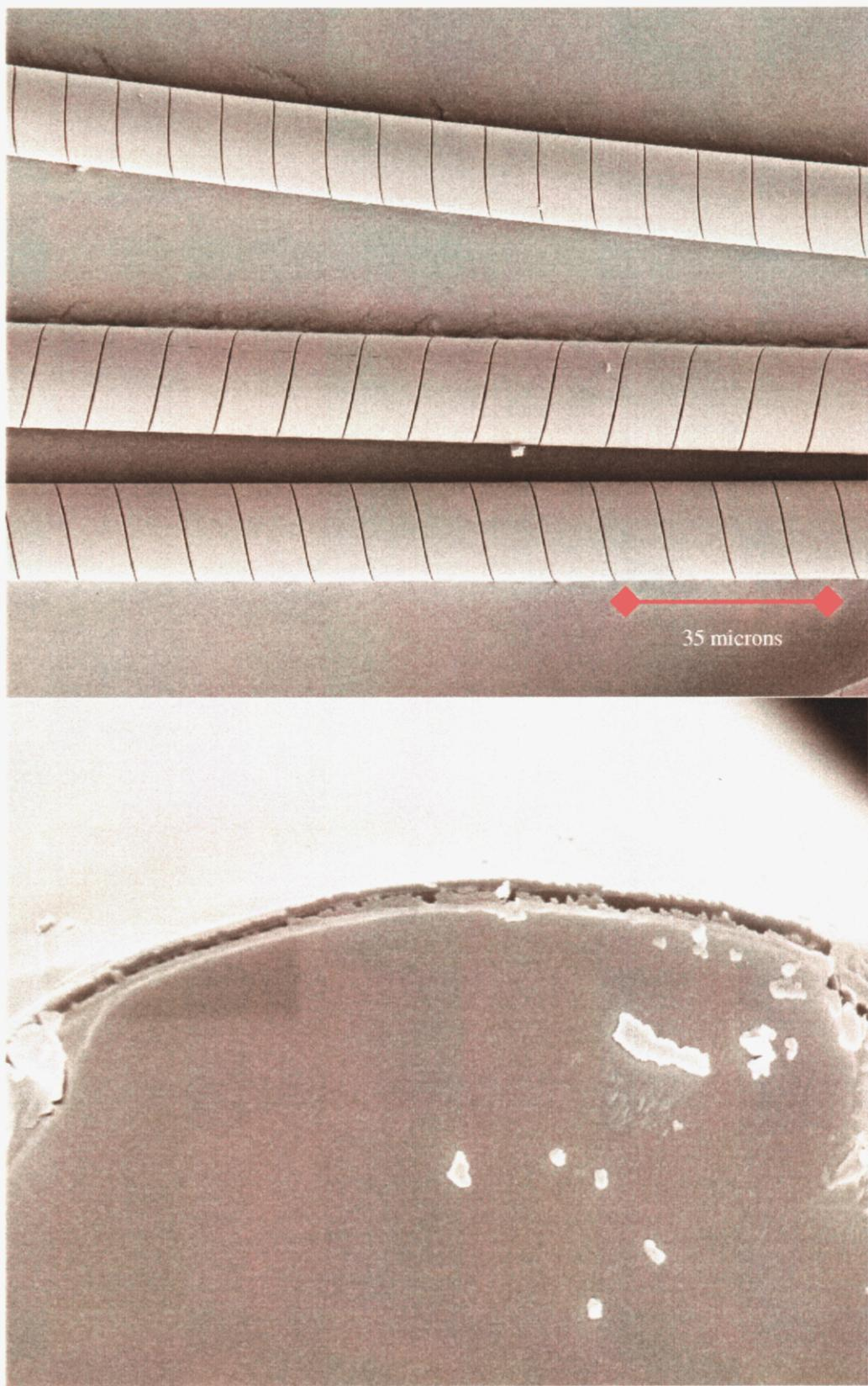
**Figure 12: SEM of acid aged aluminum borosilicate glass fibers.**
