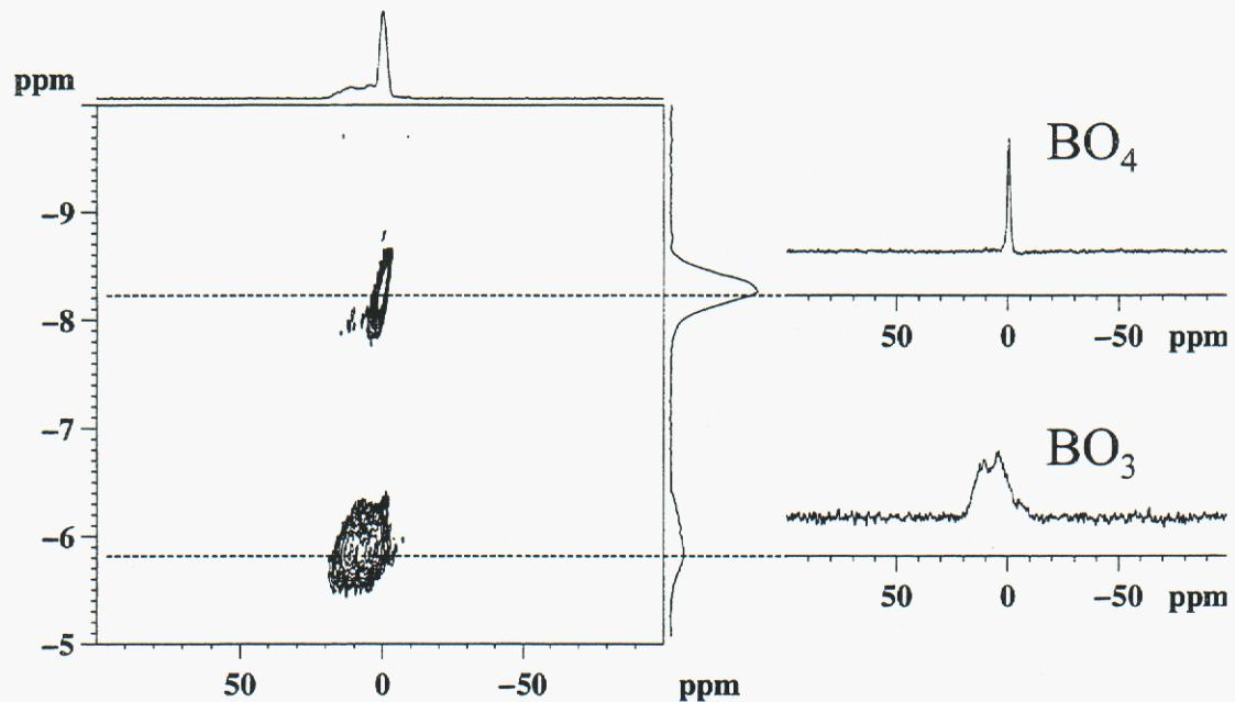
Figure 10:  $^{11}\text{B}$  MQMAS of unaged bulk aluminum borosilicate glass.
