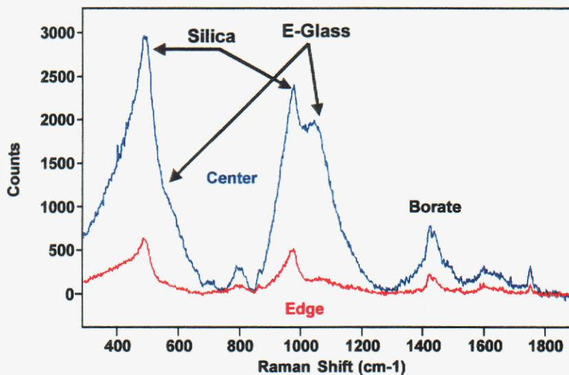
**Figure 20. Micro-Raman spectra of inner locations on the end of another aged fiber, which appears to be partially leached at its center**
