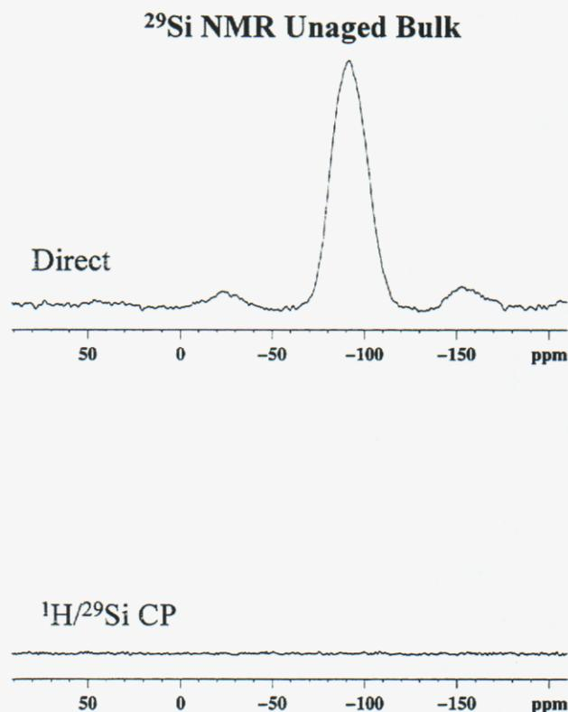
**Figure 5:**  $^{29}\text{Si}$  MAS NMR of unaged bulk aluminum borosilicate glass.
