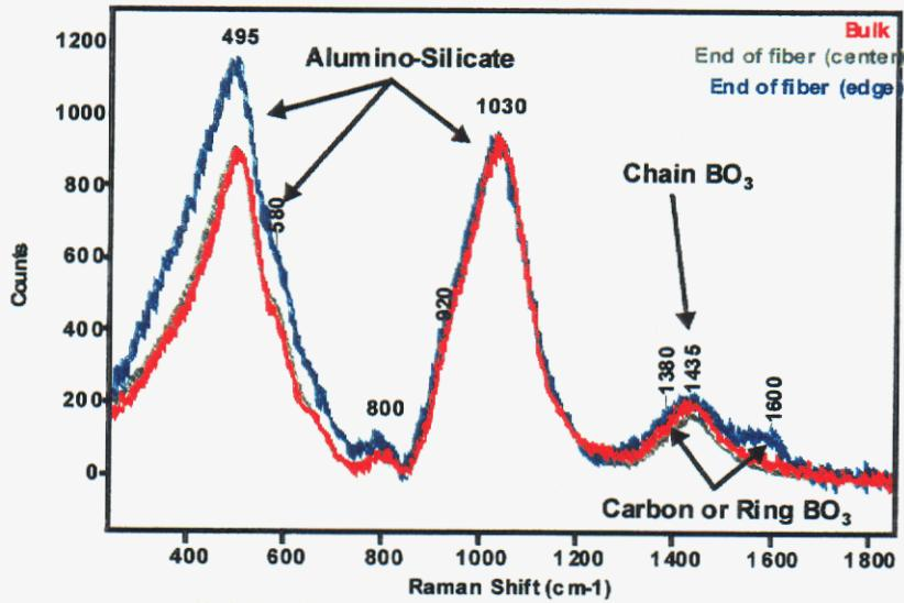
Figure 4: Raman spectra of aluminum borosilicate glass (bulk and fiber).
