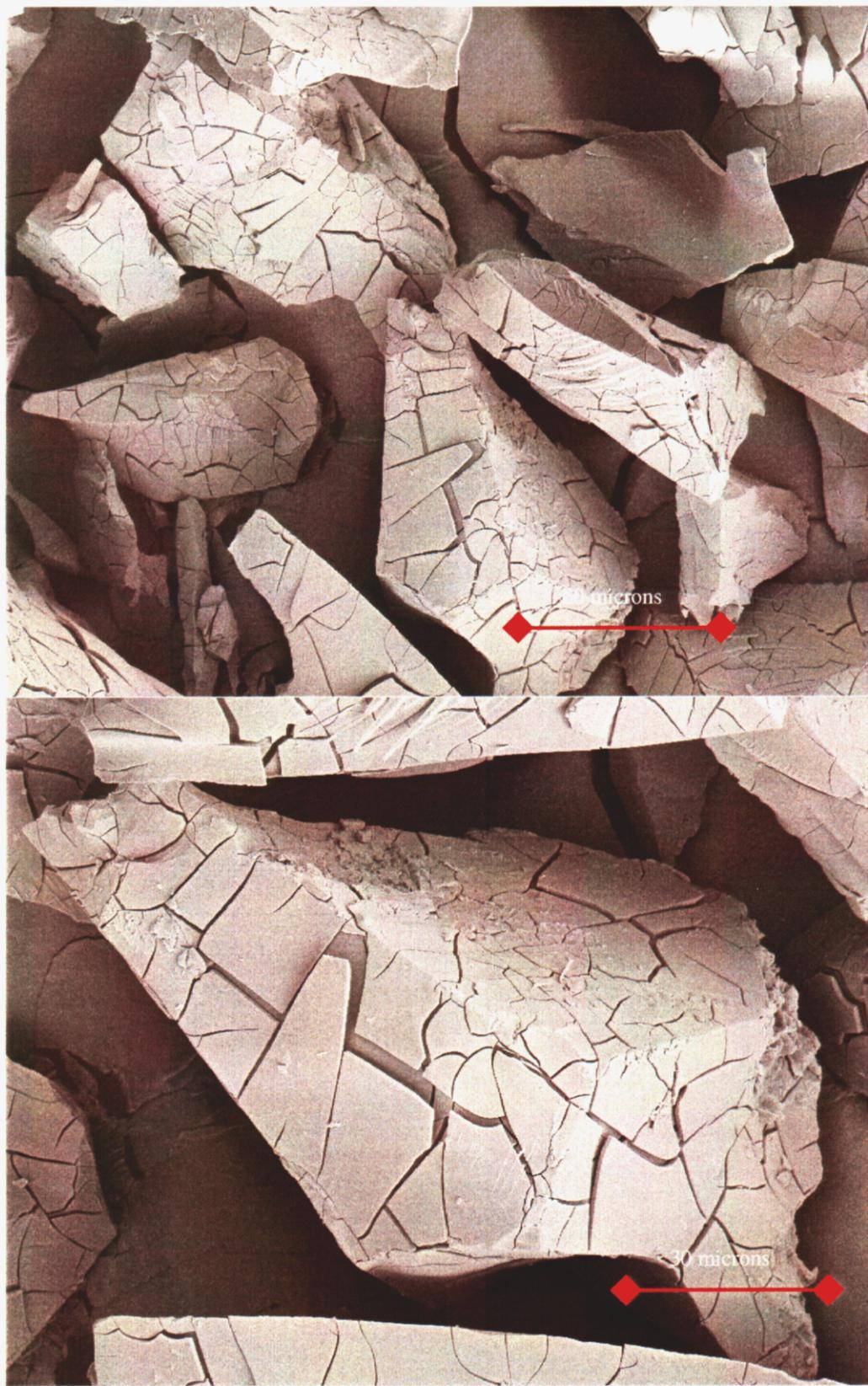
**Figure 11: SEM of acid aged bulk aluminum borosilicate glass.**
