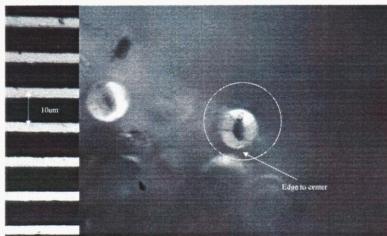
**Figure 17. Micrograph of aged fiber end.**
