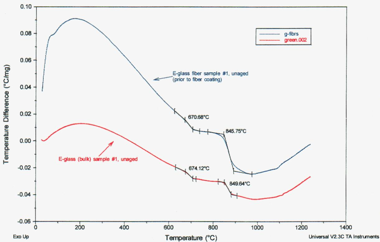
Figure 1: DTA of unaged bulk and fiber JM glass samples.
