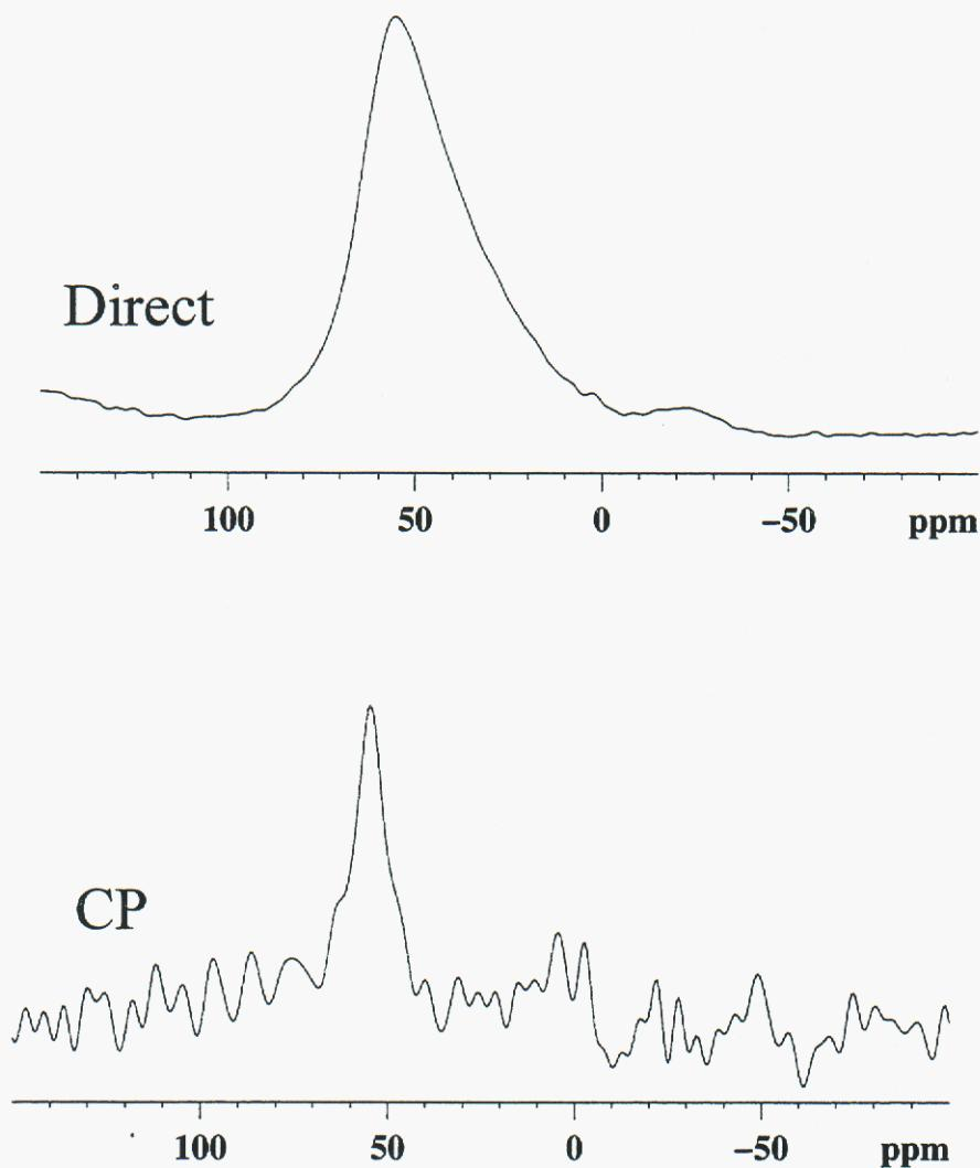
Figure 24:  $^{27}\text{Al}$  CPMAS NMR spectra of acid aged aluminum borosilicate glass.
