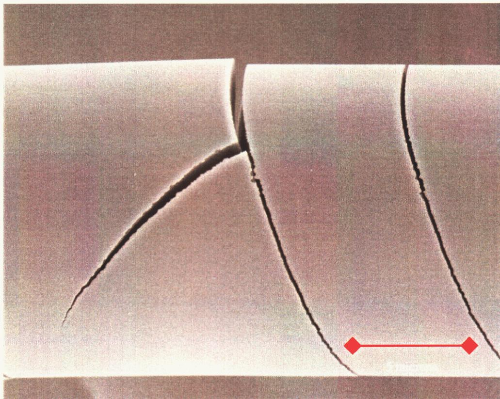
**Figure 13: SEM image of stress cracks in aged aluminum borosilicate glass fibers.**
