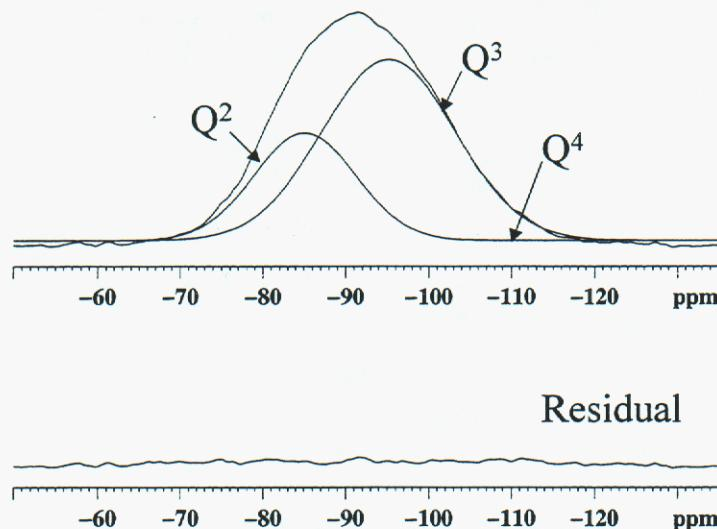
**Figure 6: Deconvolution analysis of  $^{29}\text{Si}$  MAS NMR - unaged bulk.**
