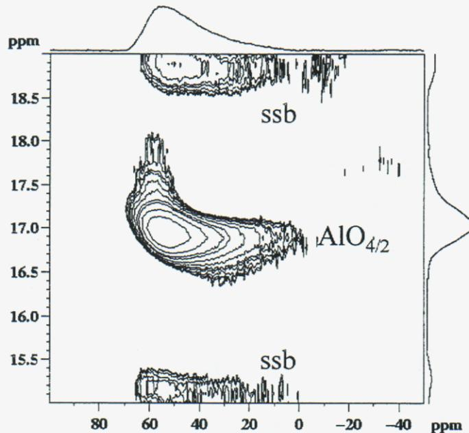
**Figure 7:  $^{27}\text{Al}$  MQMAS of unaged bulk aluminum borosilicate glass.**
