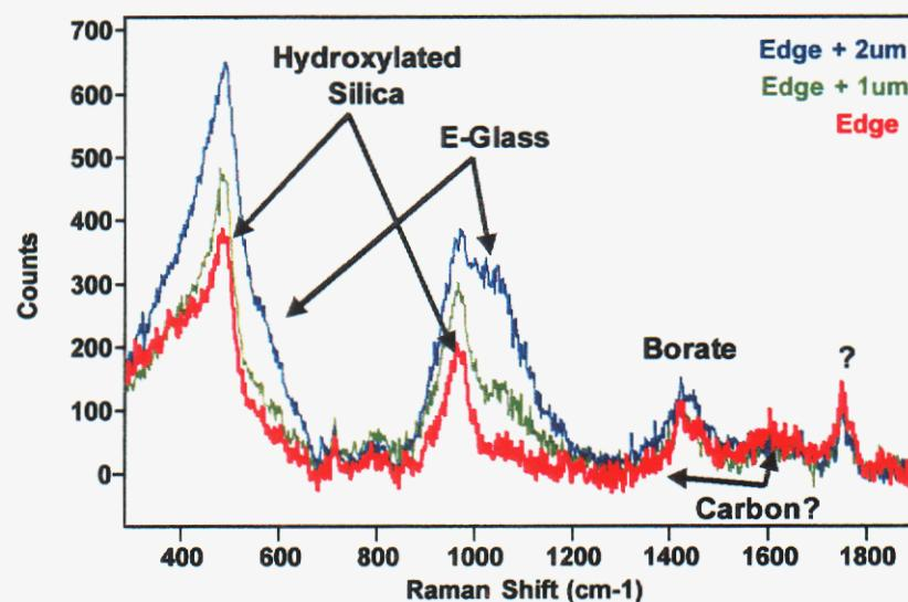
**Figure 18. Micro-Raman spectra of outer locations on the end of aged fiber.**
