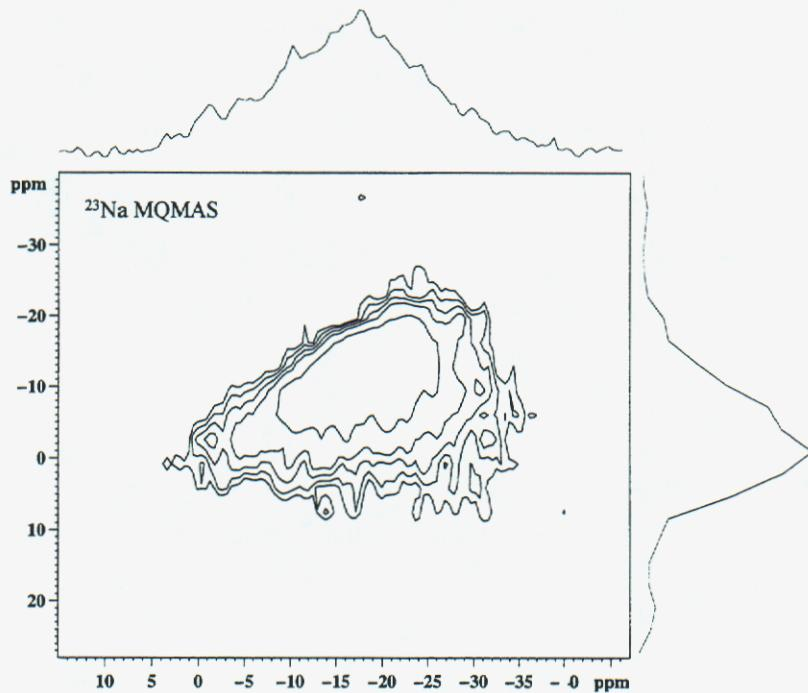
Figure 8:  $^{23}\text{Na}$  MQMAS of unaged bulk aluminum borosilicate glass.
