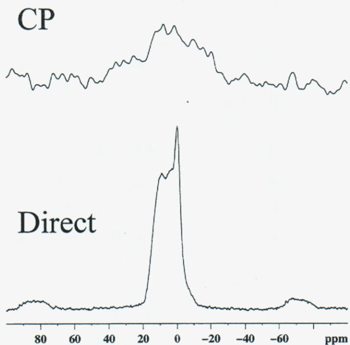
Figure 25:  $^{11}\text{B}$  CPMAS NMR spectra of acid aged aluminum borosilicate glass.
