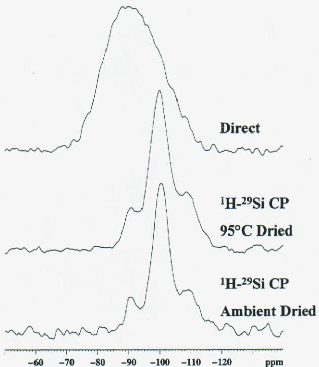
Figure 21:  $^{29}\text{Si}$  MAS NMR of acid aged bulk aluminum borosilicate glass.
