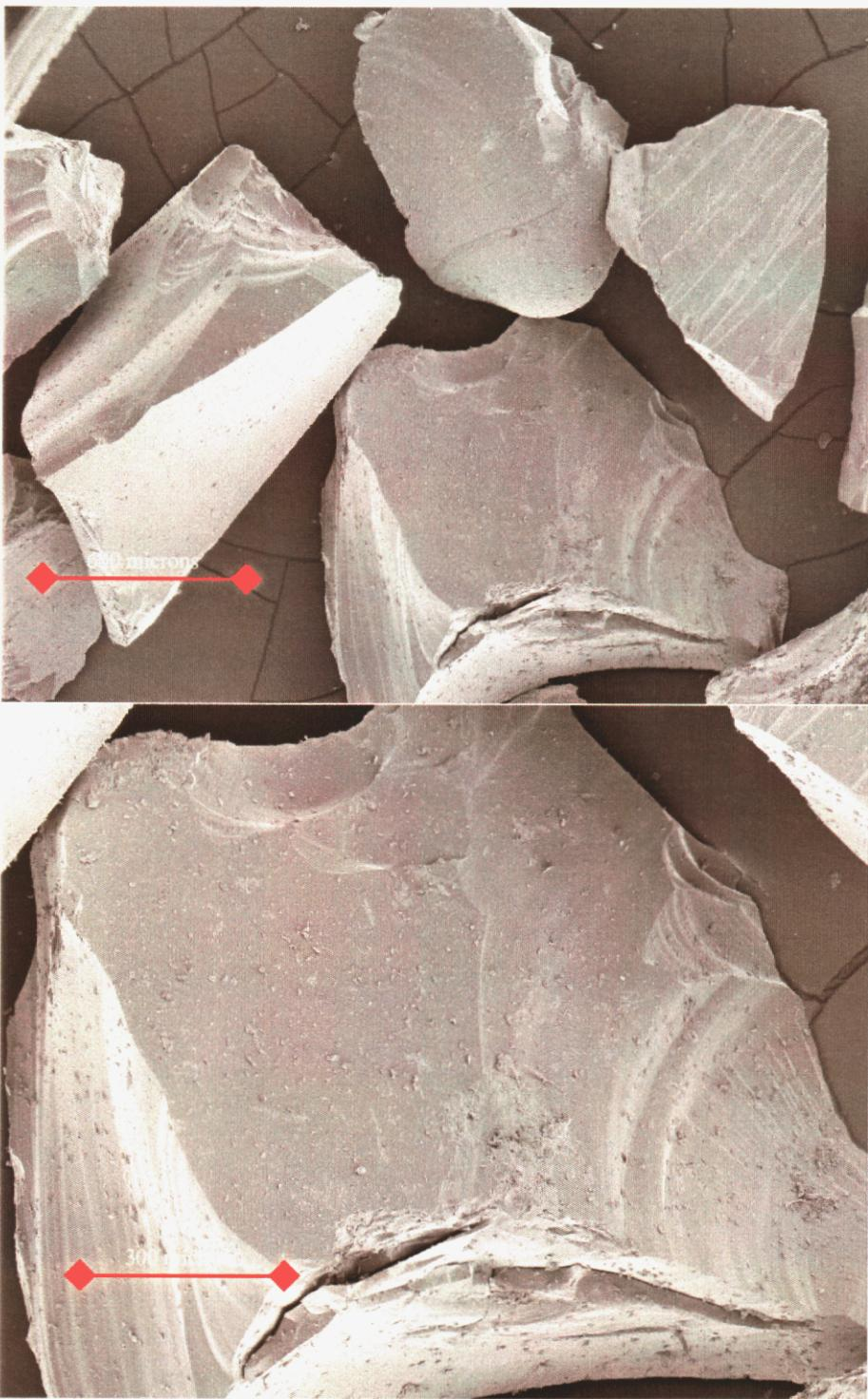
**Figure 2: SEM images of unaged bulk glass samples (400 sieve).**
