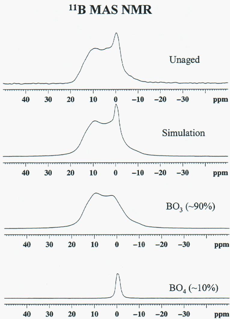
**Figure 9:**  $^{11}\text{B}$  MAS NMR of unaged bulk aluminum borosilicate glass.
